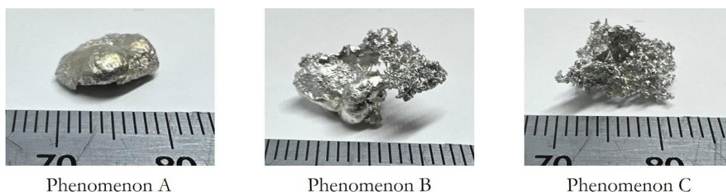
Figure 3-21: Morphology of debris from three typical phenomena in tests.
