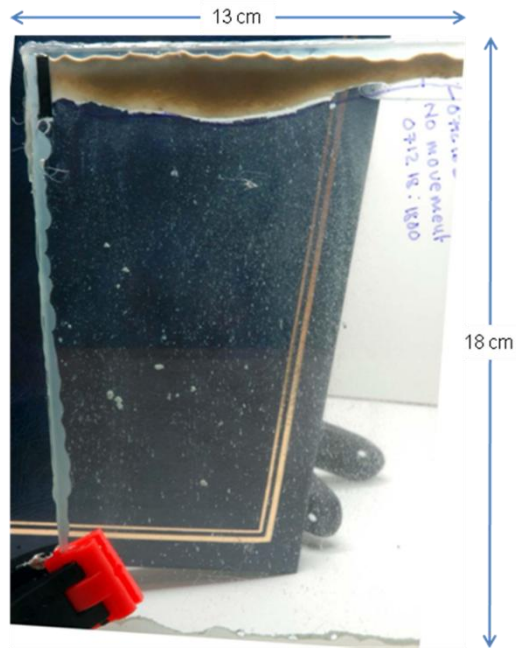
Figure 2.3.1_1. Artificial water-filled fracture formed from two glass plates with a layer of brown bentonite between the plates at the top (Neretnieks, 2009).
