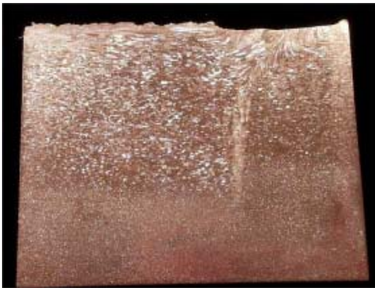
Figure 9. Closing of the keyhole is done with a linearly defocusing of the focal spot during about 10 seconds and a decrease of the power at the same time (from Outokumpu).
