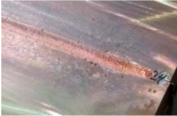
Figure 10. A view of the EB welds after a subsequent surface smoothing run (from Outokumpu).
