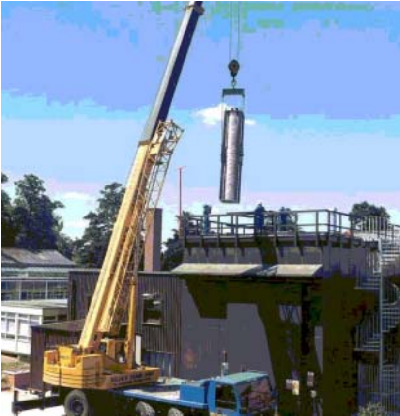
Fig 7. A 5m long, 1m diameter copper canister assembly, being lowered into TWI's Reduced Pressure Facility at Abington, Cambridge.
