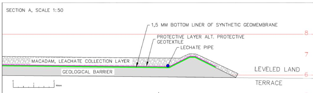
Figure 14. Design of the bottom structure.
