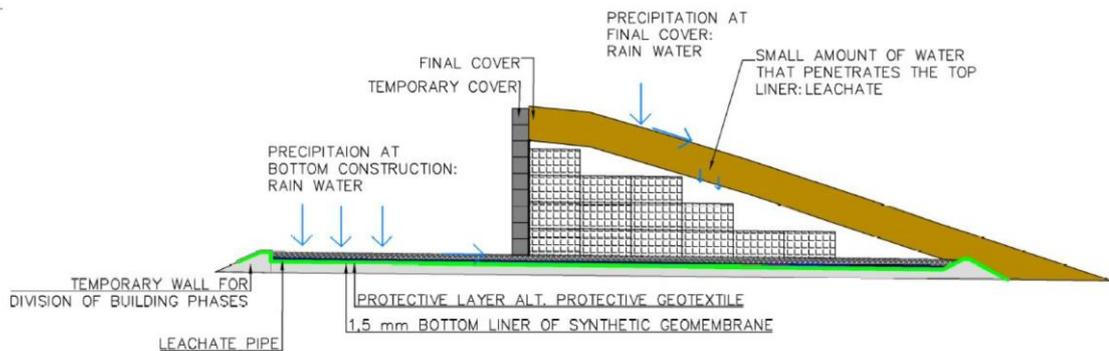
Figure 16. Principle sketch of phased expansion and temporary closure.
