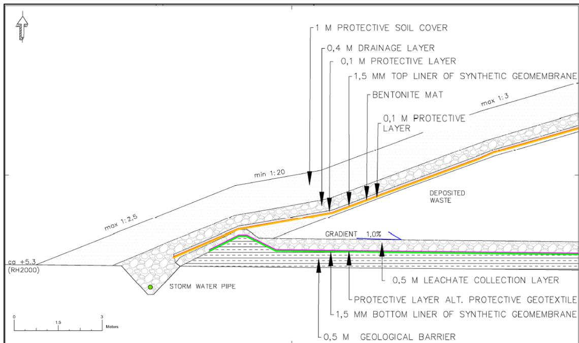
Figure 18. Cross-section of the ground repository's construction, including design of the toe of slope. Note that this sketch might be subject to minor changes regarding the stated measurements.
