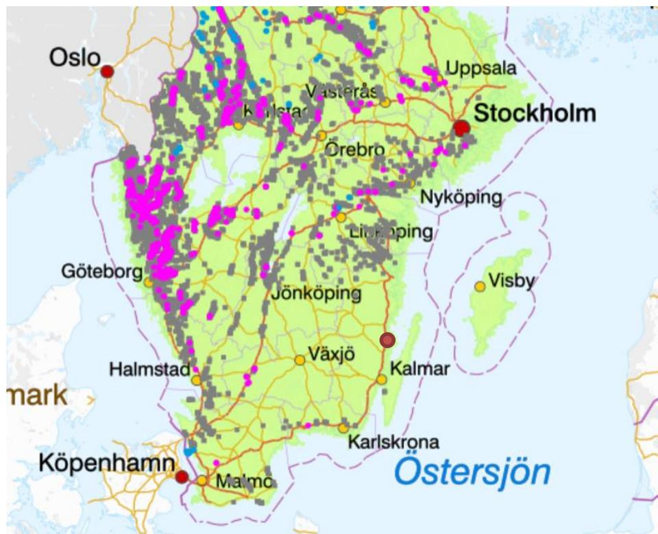
Figure 6. Traces of occurred landslides and ravines in loose soil layers. Analysis based on detailed height data and information from SGU soil databases. SGU, 2021. [6]
