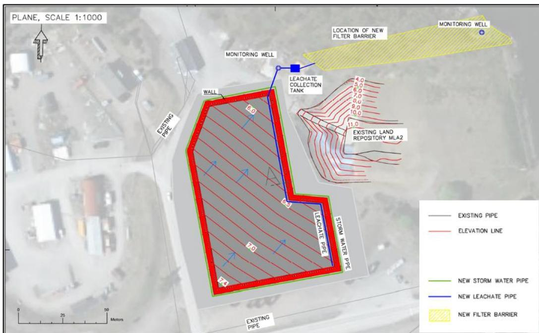
Figure 20. Bottom structure and system for management of leachate.
