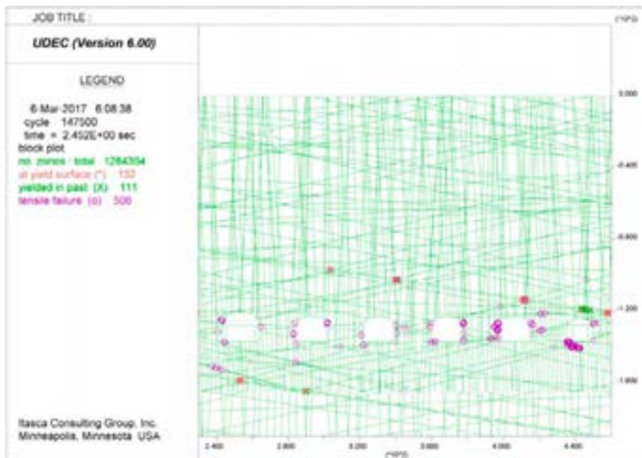
Figure A184. UDEC results after construction and backfilling stages, showing yielded elements for SFR 3, DFN 3-4.
