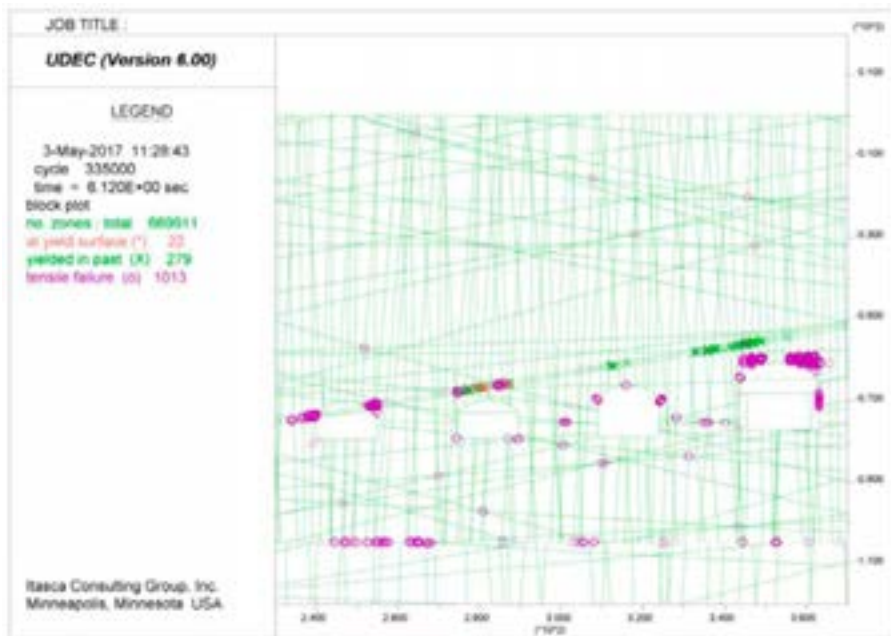
Figure A96. UDEC results after strength degradation and permafrost melting at Year 21,000, showing yielded elements for SFR 1, DFN 1-2.
