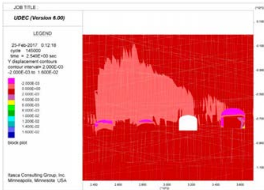
Figure A24. UDEC results after construction and backfilling stages, showing vertical displacements for SFR 1, DFN 1-2. Displacements are in units of metres, with positive up.
