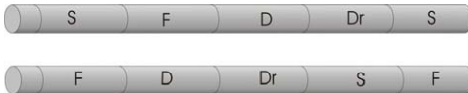
Figure 2.1. Example of cyclic sampling of the cores where the (S) is the specimens subject to saline environment, (F) formation water, (D) distilled water and (Dr) are dry conditions.
