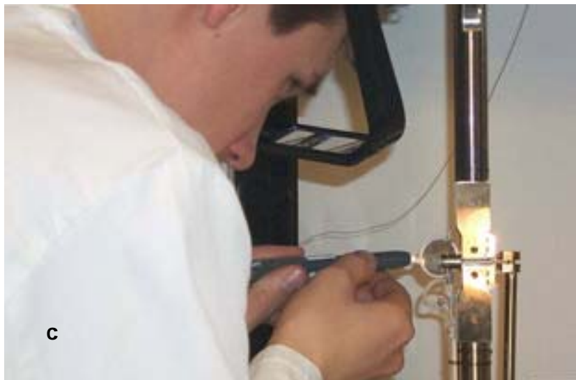
FIG. 7. The PLT-fixtures for specimen length of 9 mm and 13 mm (a); electrical connections for potential drop measurements on the PLT-specimen (b); visual control of crack extension during fatigue pre-cracking (c); and schematic view of the pull rod assembly placed into the furnace together with the displacement transducer (LVDT) attached to the fixture mouth (d). The fixture for specimens PLT-13 is shown without ceramic coating (see Fig.7a).
