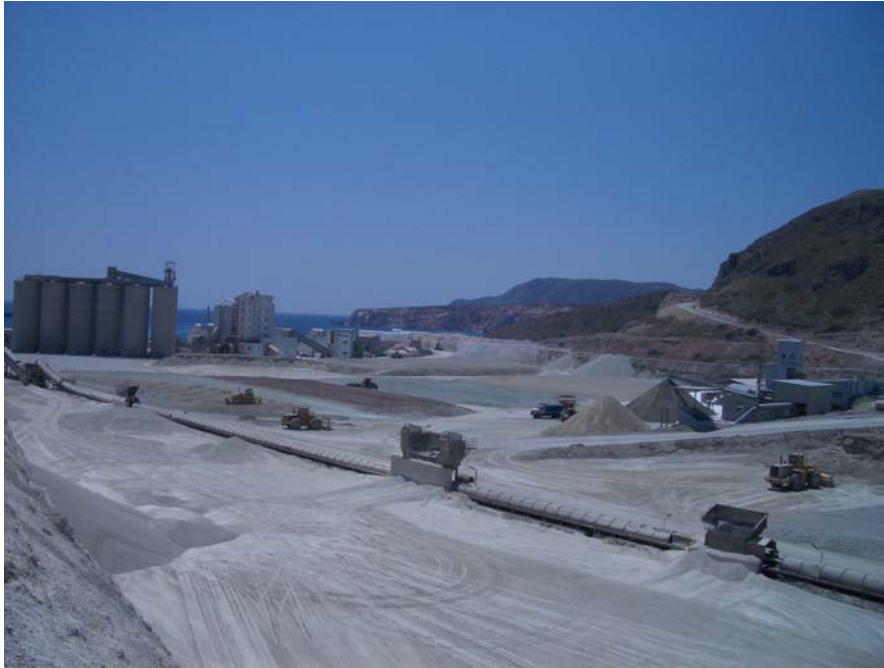
Figure 2. Sun drying of bentonite at the Greek island Milos, which is one of the largest producers in Europe. The material Deponit CaN (Silver & Baryte Ores Mining Company) originates from this facility.
