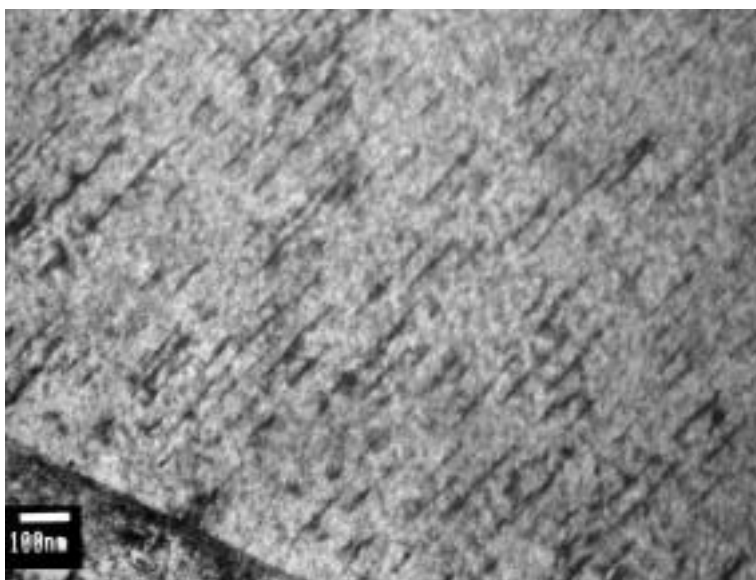
Figure 6. c component damage in the low burnup specimen. The c -axis is perpendicular to the direction of the apparent line segments. 65000x.
