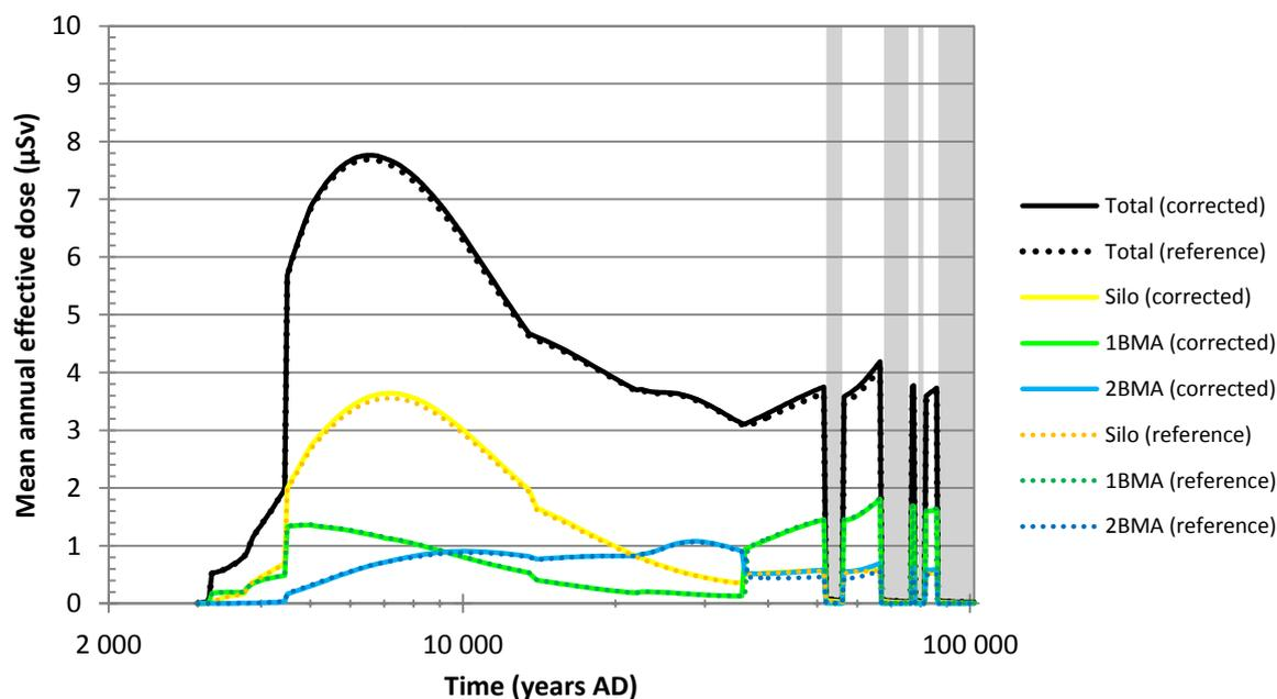
**Figure 2-1.** Arithmetic mean of the annual effective dose to the most exposed group, for releases from the entire extended repository and contributions from 1BMA, 2BMA and Silo waste vaults, in the global warming calculation case. The unshaded areas correspond to temperate climatic conditions and the grey shaded areas to periglacial conditions with continuous permafrost. The dotted lines show the result as calculated in the reference case.
