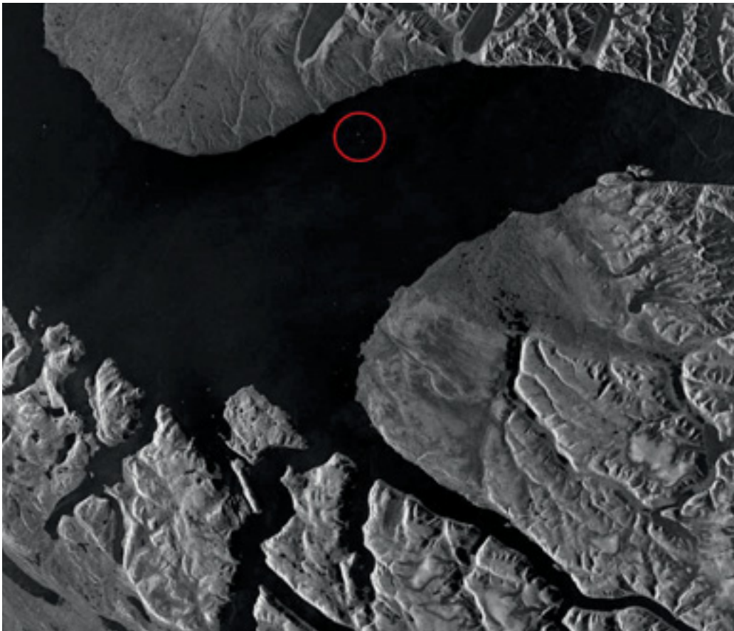
Figure 7.11. SAR-picture from the Canadian satellite RADARSAT-1. Dark areas are ice and light areas are land. The bright spots within the ring are a group of students from an ice exploration ship (from [20]).
