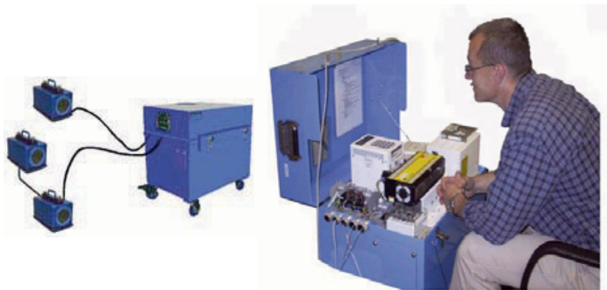
Fig. 7.6. The SDIS system with 3 DCM14 cameras connected (left) and the server equipment (right).
