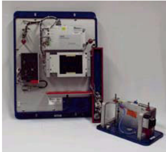
Fig. 7.9. A DSOS system with the casings of the camera (right) and the read-out unit (left) removed.
