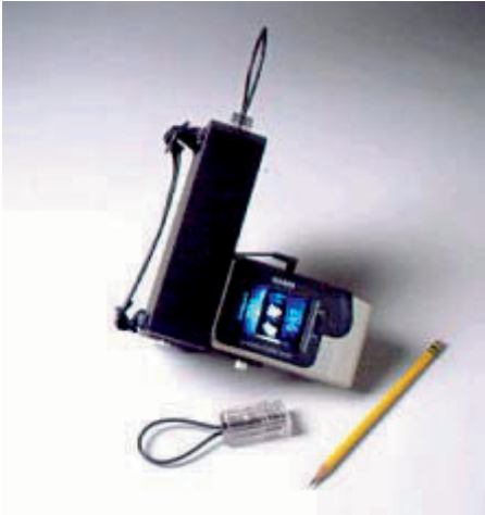
Fig. 7.3. The so-called COBRA III imaging system. The seal is at the bottom of the picture and above that is the read-out equipment. The picture is copied from ref. [21].
