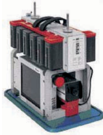
Fig 7.7. The ALIP system with viewing screen (left) and battery package (on top).
