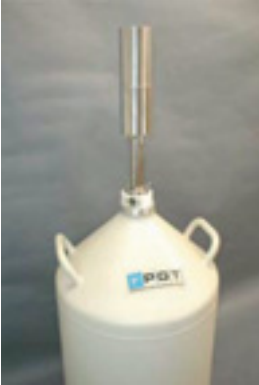
Figure 3.12. A typical Germanium detector with its dewar vessel.
