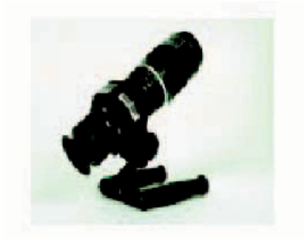
Figure 5.5. The ICVD. The UV-transparent objective is to the right and the eyepiece to the left. The instrument stands on the two handle bars. (Photo: IAEA).
