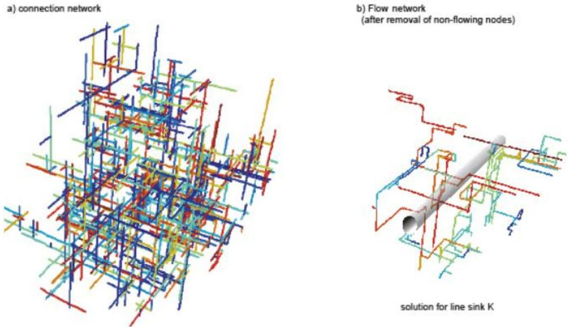
**Figure 3.** Example of how a sparse network of connections, shown in (a) is reduced to an even sparser flow network shown in (b). Note that the modelled system is a cylinder of 90-m diameter as the outer boundary and the drift is 4-m diameter as the inner boundary (Black et al., 2006). Different colors represent different networks.
