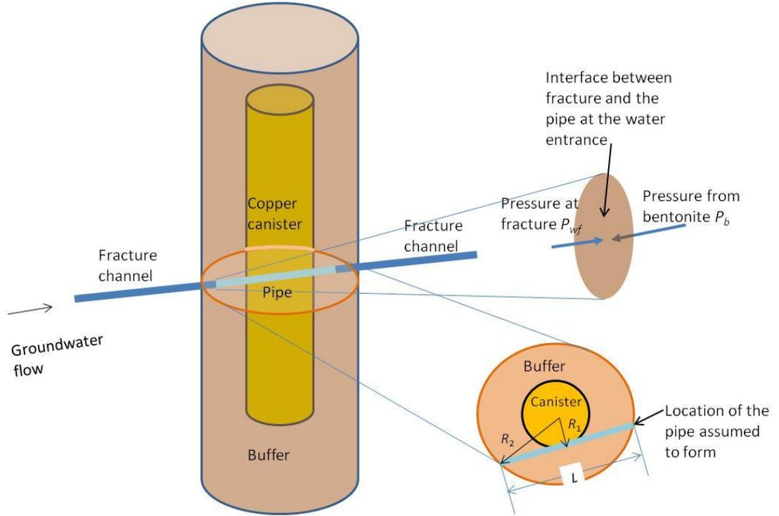
**Figure 1.** Illustration of a hypothetical “wormhole” in the buffer used in the assessment. The top right small cross section illustrates pressure balance before the pipe forms. The bottom right cross section illustrates the pipe that was assumed to form and remain open.  $R_1$  is the radius of the copper overpack [m],  $R_2$  is the buffer outer radius [m], and  $L$  is the length of the hypothetical pipe.
