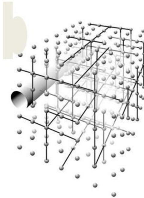
**Figure 2.** An example of Sparse Channel Network generated by 3D lattice network model. Channels are represented by dark lines, i.e., the connected bonds at the lattice corners (Black et al., 2013).
