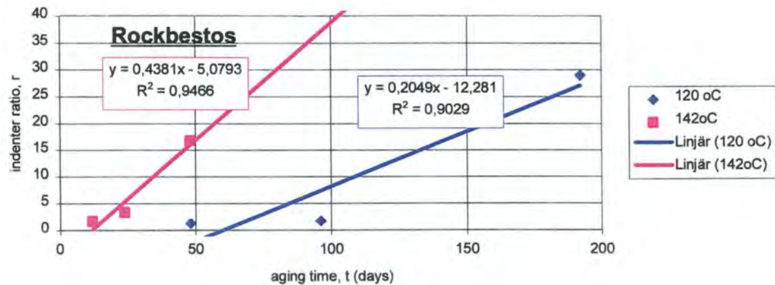
Diagram 5.3 Indenter ratios of thermally aged cables, kab d (sealed)
