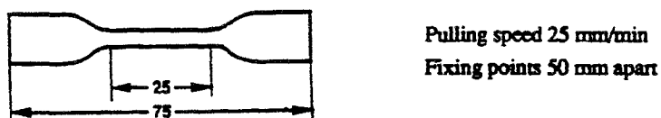
Figure 4.2 Test specimen used for elongation at break measurement
