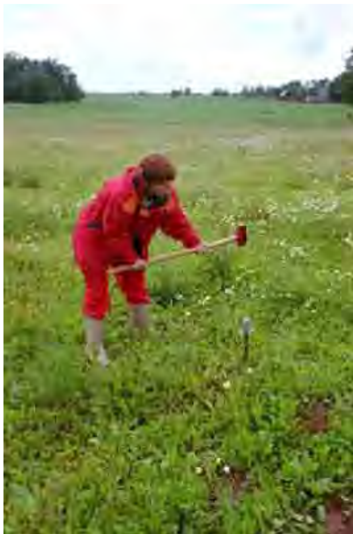
Figure 11. Krista Täht hammering the steel pipe to sample soil air.
