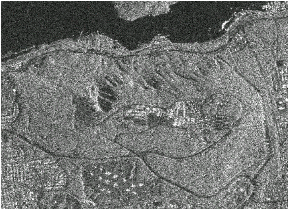
Figure 7. RADARSAT data, Fine Beam Mode sample. Roads and other infrastructure are easily distinguishable. ©Canadian Space Agency/Agence spatiale canadienne.
