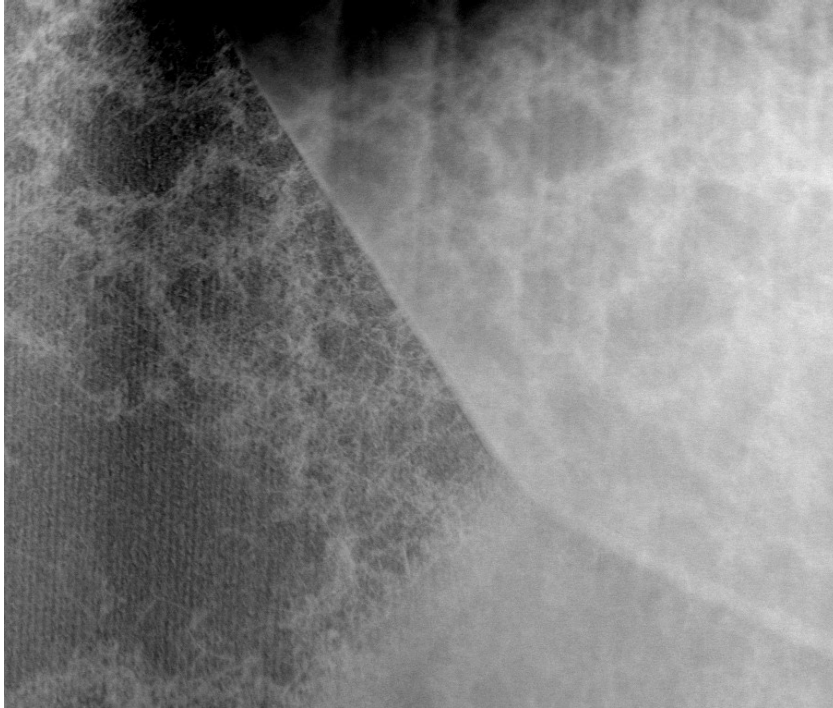
Figure 8. TEM (HAADF) image of three GBs and a triple point in OFF (Titan).
