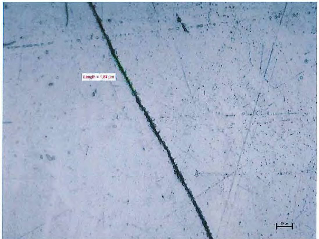
Micro-photograph of the “defect” showing the distance between the base material and insert to be approximately 2 \mu\text{m} .
