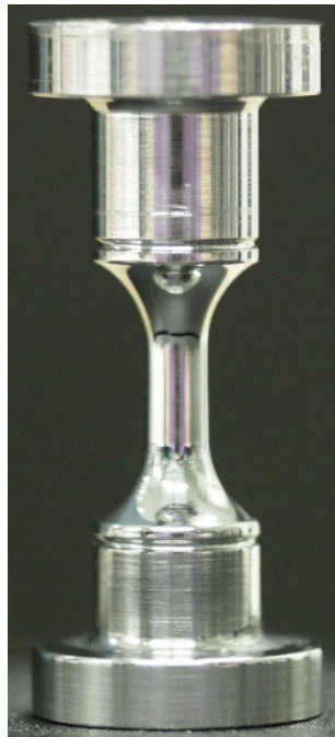
Figure 3 : Alternative specimen design with reduced gauge length and low strain (larger diameter) region for reference of potential drift.
