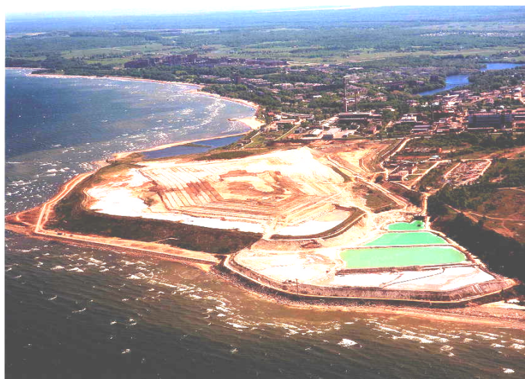
A similar aerial view from 2004 over the Sillamäe site. The shoreline and the dam are reinforced and quite a large part of the dam is now covered.
