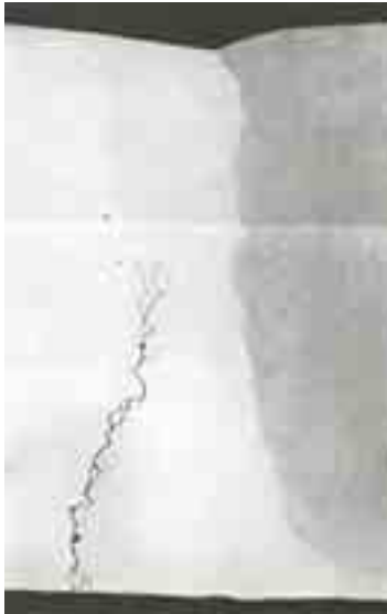
Figure 6-8 Typical orientation in the through thickness direction of an IGSCC in austenitic stainless steels
