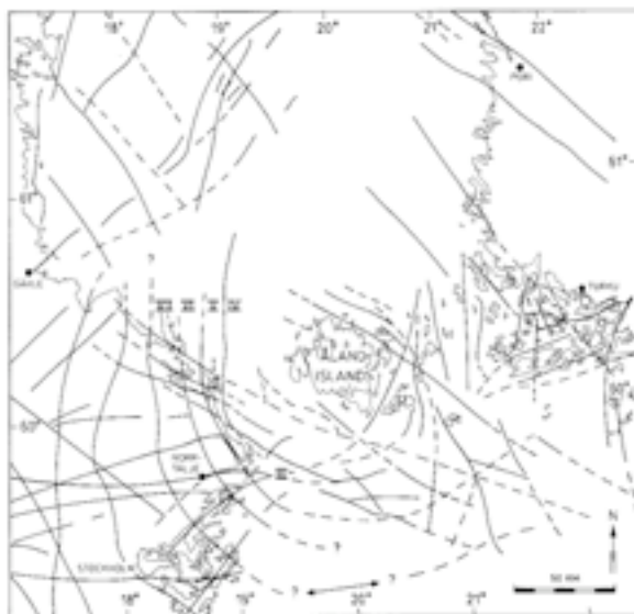
Figure 1-3. Structural map emphasising the concentric tectonic structures centred on Åland, an area of approximately 1.6 Ga old rapakivi granites (Söderberg 1993).
