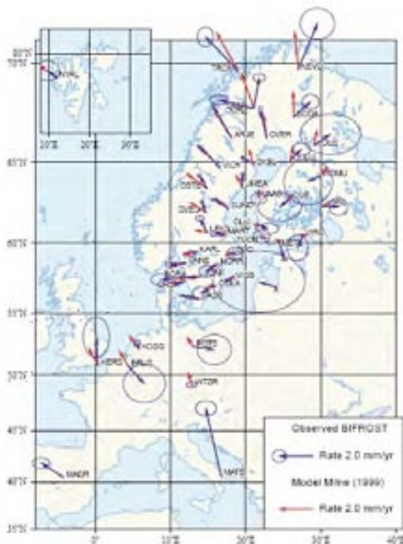
Figure 2-14. Predicted present day horizontal velocities from the visco-elastic earth model and observed motion estimated from the BIFROST network; dark blue arrows and confidence circles (Scherneck et al. 2001, cf. Fig. 2-12c).
