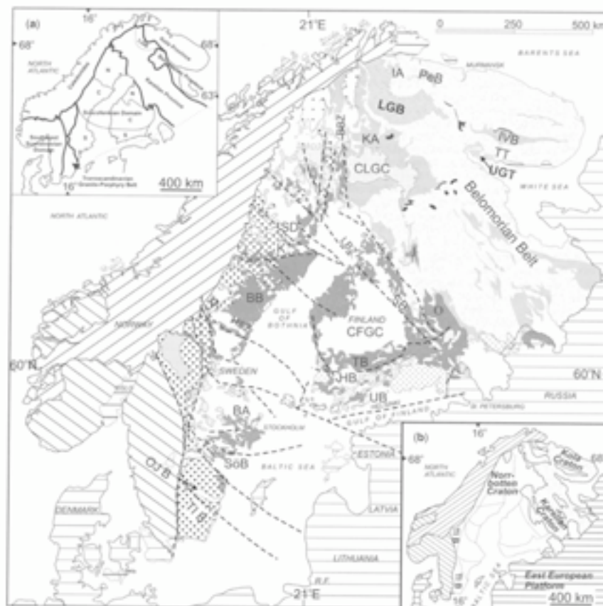
Figure 4a. Simplified geological map of the Fennoscandian Shield, based on Kostinen et al. (2001). The shear zones are mainly interpreted from magnetic and gravity maps (Korhonen et al. 2002). (a) major geological units of the Fennoscandian Shield, after Gaál & Gorbatshev (1987). N, Northern Svecofennian Subprovince; C, Central Svecofennian Subprovince; S, Southern Svecofennian Subprovince, (b) Archaean cratonic terranes of the Shield. Archaean units: Norrbotten craton, Kola craton, and Karelian craton, including Belomorian. Palaeoproterozoic units in Kola peninsula: IA, Inari area; PeB, Pechenga Belt; IVB, Imandra Varzuga Belt; UGT, Umba Granulite Terrane; TT, Tersk Terrane. Palaeoproterozoic units in Finland: LGB, Lapland Granulite Belt; KA, Kittilä allochthon; CLGC, Central Lapland Granitoid Complex; SB, Savo Belt; CFGC, Central Finland Granitoid Complex; TB, Tampere Belt; HB, Häme Belt; UB, Uusimaa Belt. Palaeoproterozoic units in Sweden: SD, Skellefte district; BB, Bothnian Basin; BA, Bergslagen area; SöB, Södermanland Basin, OJB, Oskarshamn-Jönköping Belt; TIB, Transscandinavian Igneous Belt. J, Jormua; K, Knaften; O, Outokumpu; R, Revsund; BBZ, Baltic-Bothnia Megashear; HSZ, Hassela Shear Zone; LBZ, Ladoga-Bothnia Bay Zone. From Korja et al. 2006.
