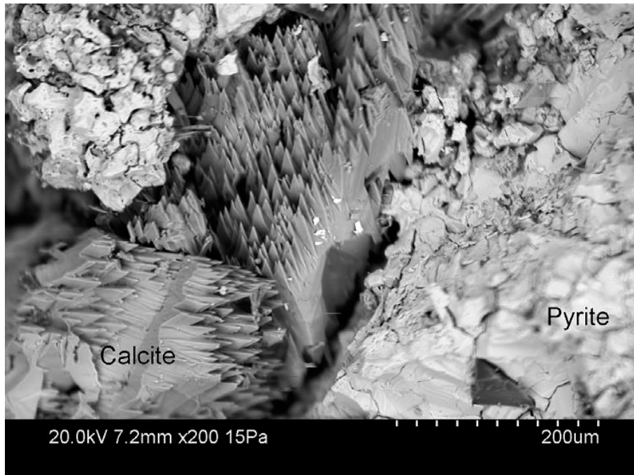
Figure 4 Backscattered electron image of calcite and pyrite crystals (from Sandström et al., 2011; page 47). Etching of calcite due to dissolution is clearly visible.
