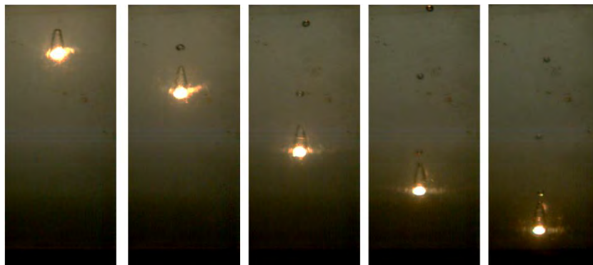
Figure 3-108: Raw snapshots depicting interaction between CeO 2 -ZrO 2 ( \Delta T_{superheat}: 100\text{K} ) and water ( \Delta T_{sub} \approx 80\text{K} ).
