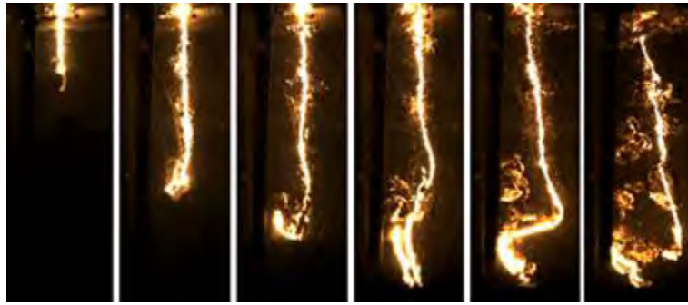
Figure 3-107: Time sequence raw snapshots depicting interaction between zirconium melt jet ( D_{jet} \approx 5\text{mm} , \Delta T_{superheat} \approx 85\text{K} ) and water ( \Delta T_{sub} \approx 83\text{K} ).
