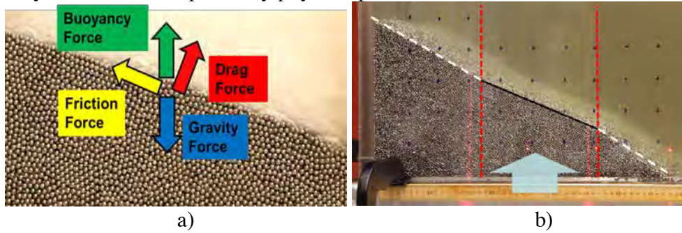
Figure 3-58. (a) Forces acting on particles near the top bed surface; (b) shape of the bed when gas is injected only under one section of the bed.
