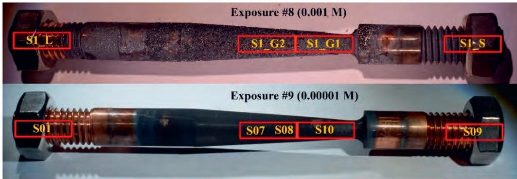
Figure 1. SSRT specimen #8 (top) and #9 (bottom) after testing. Locations and naming of TDS samples are marked with red rectangles and yellow text.
