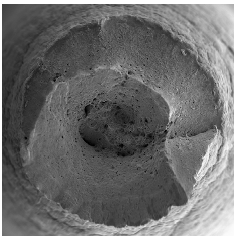
Figure B11: Fracture surface of specimen SB3, Type 316NG-H, cold work ratio = 33 %, strain rate = 1 \cdot 10^{-7} \text{ s}^{-1} .
