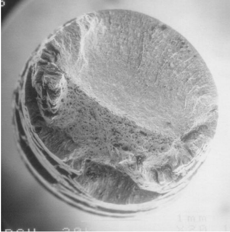
Figure B5: Fracture surface of specimen SA5, Type 316NG-L2, cold work ratio = 7.5 %, strain rate = 5 \cdot 10^{-7} \text{ s}^{-1} .
