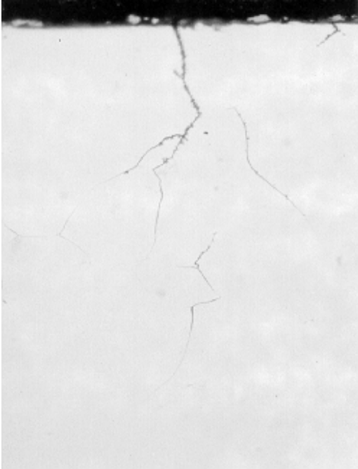
Figure C9: Cross section of test specimen CB4 (400X), Type 316NG-H, cold work ratio = 7.5 %, R = 50.
