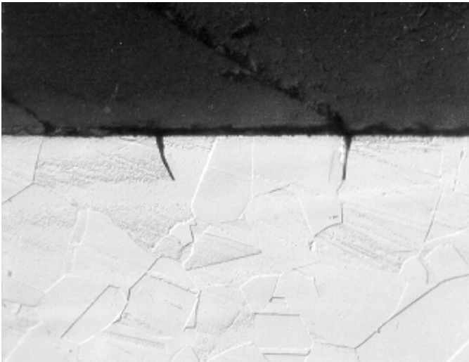
Figure C6: Cross section of test specimen CB1 (400X), Type 316NG-H, cold work ratio = 0 %, R = 100.
