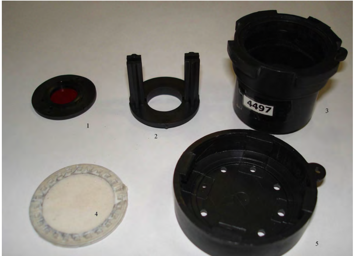
Figure 7: Alpha-track detector used in the National Radon Survey in the Republic of Kalmykia: 1 – detector holder with alpha-track detectors LR-115 Type II; 2 directing devices of the detector holder with film; 3 – plastic cup; 4 – silicon barrier (membrane); 5 – lid with holes.
