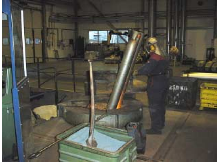
5. Feeding rack segment into melter.
