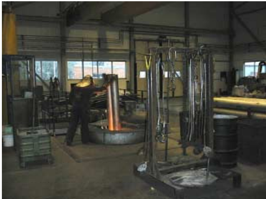
4. Feeding rack segment into melter.
