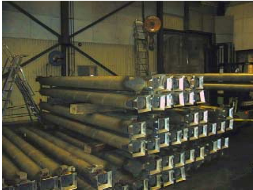
1. Segmented rack awaiting transfer to furnace.
