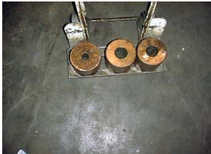
6. Moulds for samples from melt.
