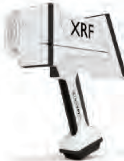
Figure 1. Schematic picture of a handheld XRF instrument
