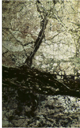
Figure 9: Micrograph of rock sample collected at Äspö, showing the effects of matrix diffusion on a mm scale – oxidising water diffusing into the rock matrix.
