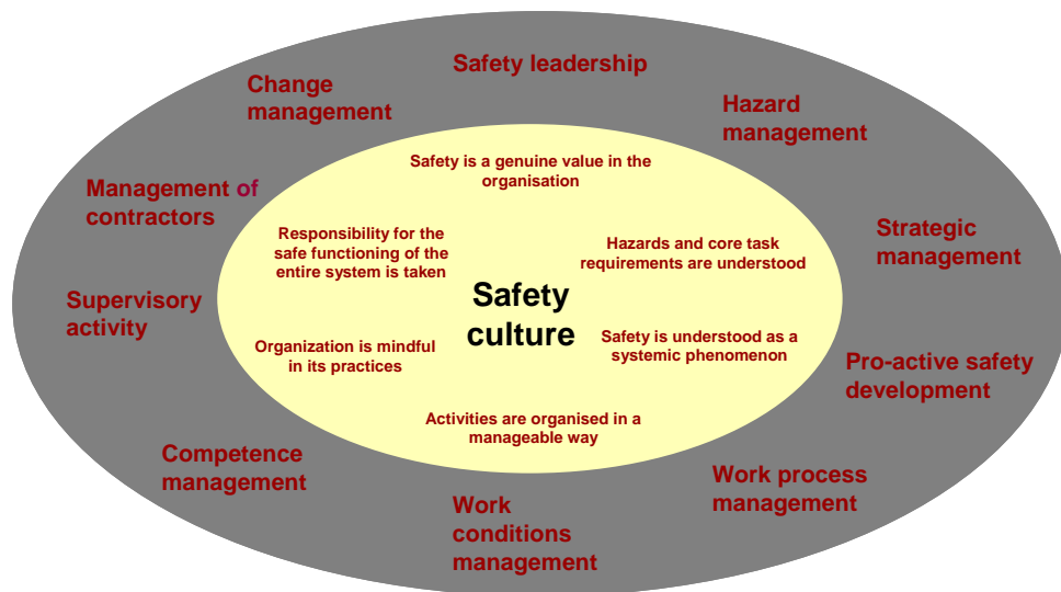
Figure 3. The DISC model describes the criteria for a good safety culture and the organisational functions necessary to develop a good safety culture in the organisation.
