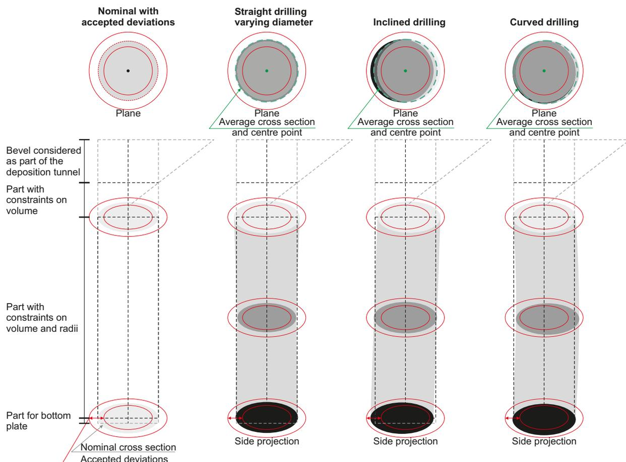
**Figure 6-1.** Some possible causes of deviations in the geometry in a deposition hole without rock fall out. All kinds of deviations can occur in the same deposition hole. The deviations are exaggerated in scale.
