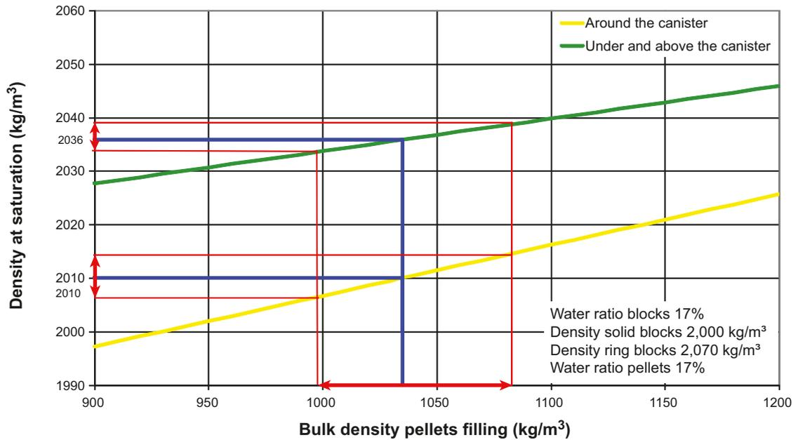
**Figure 4-5.** The calculated saturated density of the buffer (red arrows on y-axis) as function of the installed density of the pellets filling. The calculations are based on the nominal geometry of the deposition hole and nominal densities and dimensions of the blocks. (Blue line: nominal density)
