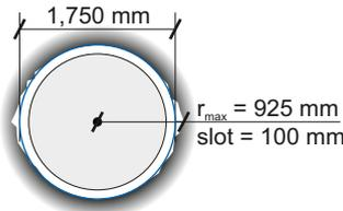
**Figure 6-2.** Increase in deposition hole radius due to spalling and rock fall out in a deposition hole with nominal diameter.
