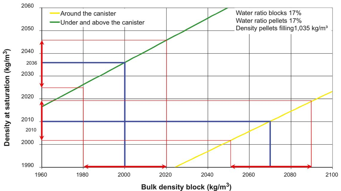
**Figure 4-6.** The calculated saturated density of the buffer (red arrows on y-axis) as function of the installed bulk density of the blocks. The calculations are based on the nominal geometry of the deposition hole and nominal density of the pellets. (Blue line: nominal density)
