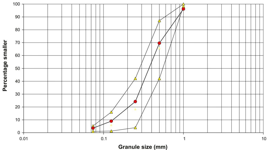
*Figure 3-1. Nominal granule size distribution and acceptable variation (based on MX-80).*
