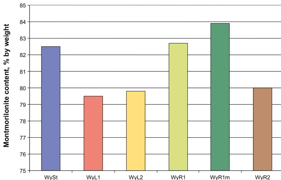
**Figure 5-5.** Results of X-ray diffraction inspections and analysis of diffraction patterns showing the montmorillonite content in the five consignments representing over 20 years of production of MX-80 bentonite /Karlund et al. 2006/. The Stripa (WySt) material represents material delivered around 1980, and the others were delivered 1995 (WyL1), 1999 (WyL2), and 2001 (WyR1 and WyR2).
