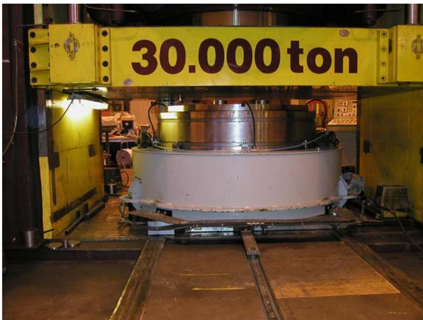
*Figure 5-7. The mould used for making ring shaped blocks for the Prototype Repository.*
