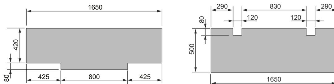
**Figure 3-2.** The nominal dimensions of the blocks placed on top (left) and beneath (right) the canister. The accepted deviation is ±1 mm for all specified dimensions.
