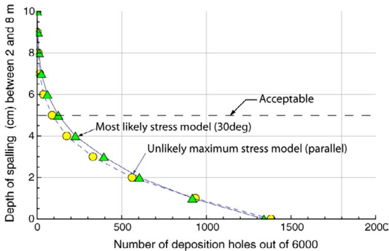
**Figure 6-4.** The number of deposition holes where the spalling reaches different depths for the “most likely” stress model with the deposition tunnel at 30 degrees to the maximum horizontal stress and the “Unlikely maximum” stress model with the deposition tunnel parallel to the maximum horizontal stress, see Section 4.3 in the **Underground openings construction report**.
