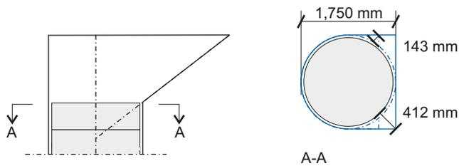
**Figure 4-3.** The cross section of the deposition hole in the area where the bevel connects to the hole. As illustrated by the dotted line the bevel will extend into the part of the deposition hole where buffer is installed.
