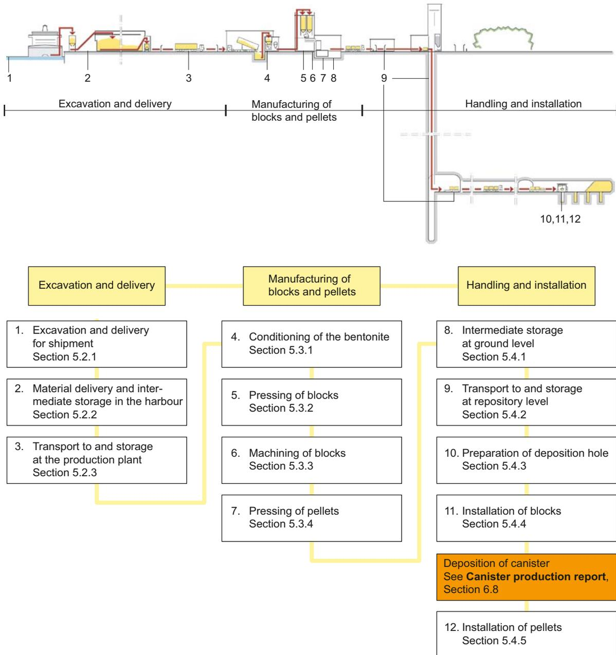
**Figure 5-1.** Upper panel: Illustration of the buffer production line from the delivery of the material to the installation in the deposition hole. Lower panel: The main parts of the buffer production line (yellow) and flow chart for all stages, including references to the numbers in the illustration and sections in the text where they are described.
