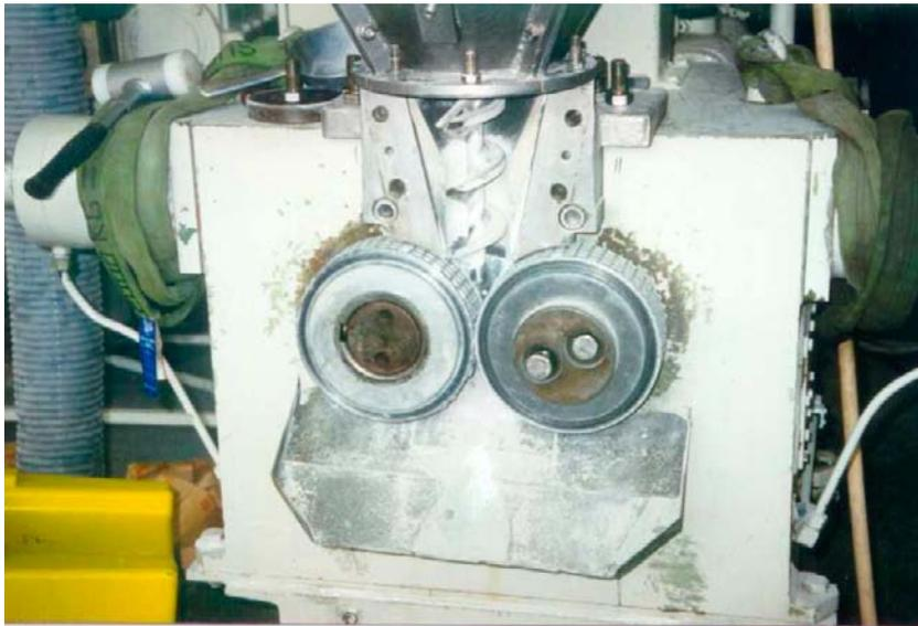
*Figure 5-10. A machine for pressing of briquette shaped pellets (BEPEX test equipment).*
