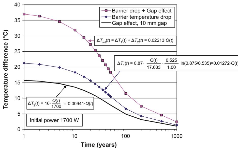
**Figure 4-9.** Evolution of the temperature difference  $\Delta T_{tot}$  for a reference case with a thermal conductivity of the buffer;  $\lambda_{b(eff)} = 1.00 \text{ W/(m}\cdot\text{K)}$ , and with gap effect scaled to the Prototype hole #6 /Hökmark et al. 2009/.
