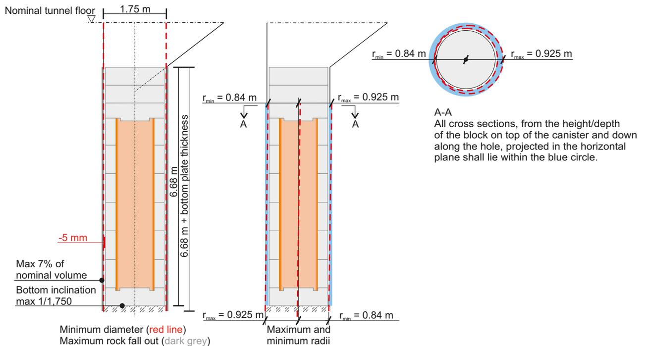
**Figure 2-1.** Nominal deposition hole geometry (black thin line) and acceptable deviations in geometry (red dotted line). The scale of the deviations in section A-A is enlarged with a factor of two. The acceptable deviations concern the part of the deposition hole where the buffer is going to be installed. The top of the deposition hole is designed with respect to operational requirements.
