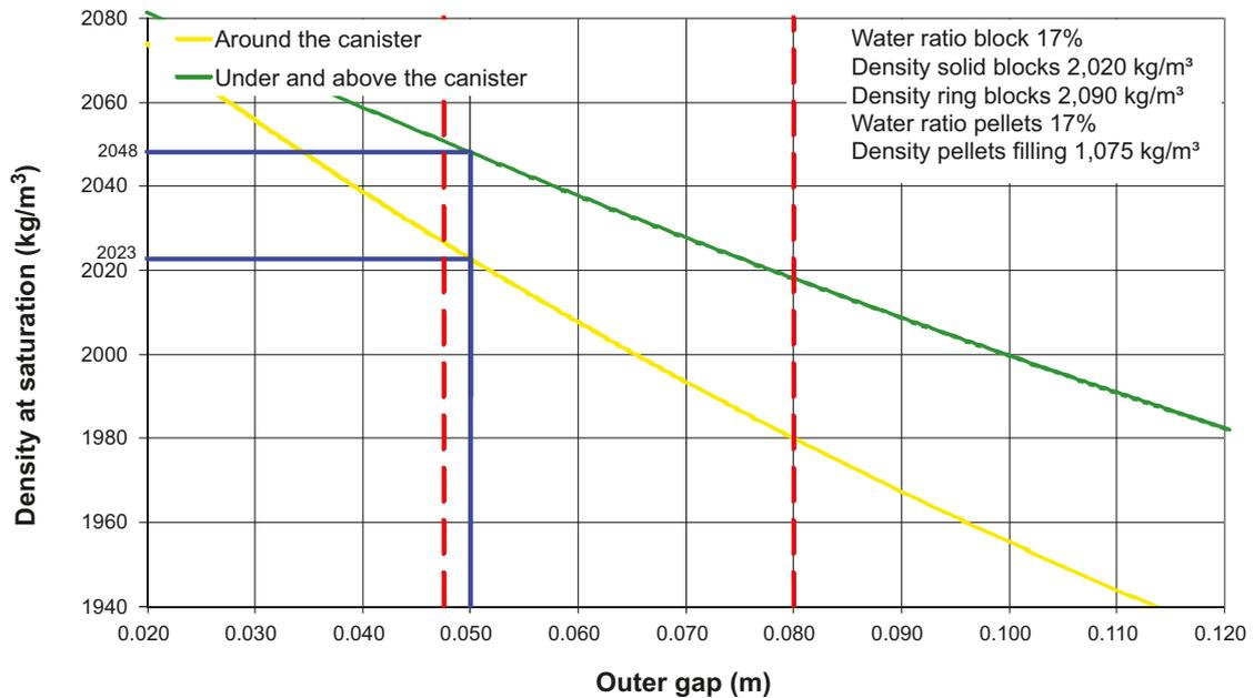
**Figure 4-8.** The calculated saturated density of the buffer as function of the width of the pellet filled gap between the bentonite blocks and the wall of the deposition hole. Upper panel: Assuming minimum density of the buffer blocks and pellets. Lower panel: Assuming maximum density of blocks and pellets. (Blue line: nominal gap.) The red dotted lines illustrate the maximum accepted area of the cross section which exceeds the nominal with 7.0%.
