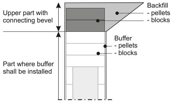
**Figure 5-13.** The upper part of the buffer and the connection to the backfill in the deposition tunnel. The two dark grey blocks are made of buffer material but are regarded as a part of the backfill. The upper part of the deposition hole down to the level where the buffer is installed is regarded as a part of the deposition tunnel.
