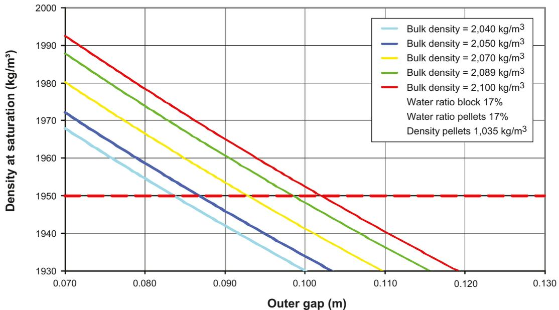
**Figure 6-3.** The density at saturation for the buffer at the level of the canister as function of the width of the pellets filled outer gap. The calculations are made assuming different bulk densities on the ring shaped blocks.
