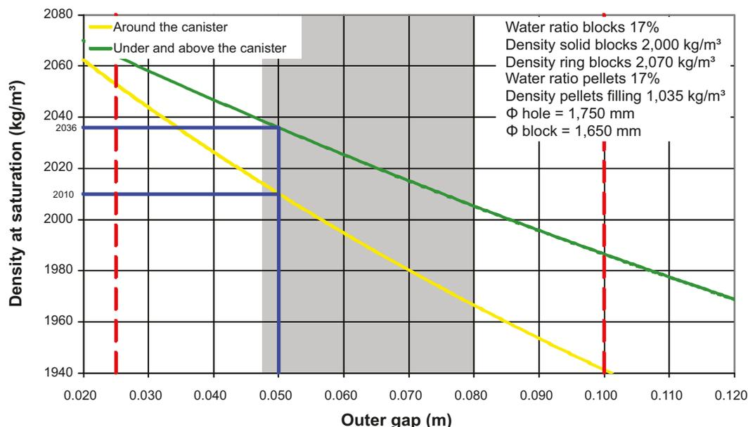
**Figure 4-1.** The calculated saturated density of the buffer as function of the width of the pellet filled gap between the bentonite blocks and the wall of the deposition hole. (Blue line: nominal gap. Red dashed lines: acceptable width of gap. Grey shaded area: corresponding to minimum diameter (1,745 mm) and diameter (1,810 mm) of a circle with maximum acceptable area).
