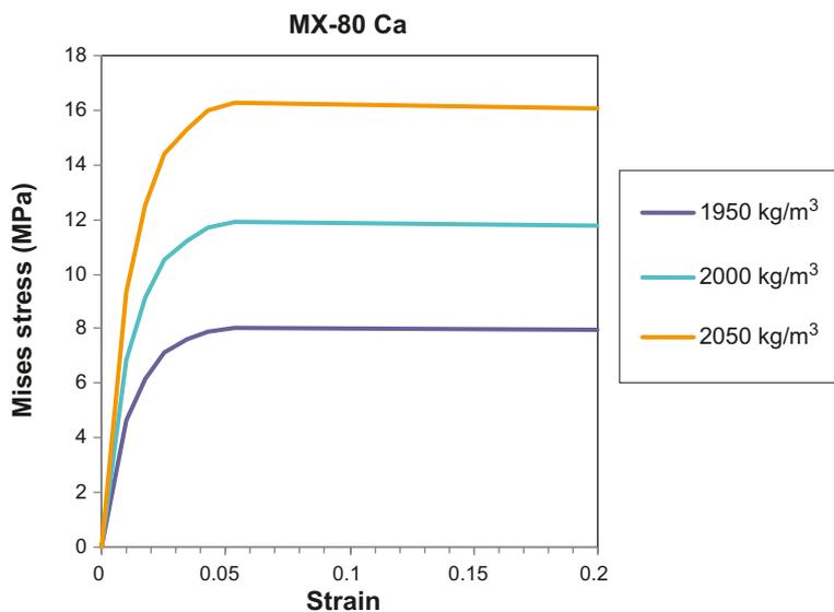
**Figure 4-11.** Dimensioning stress-strain relation for the buffer based on MX-80 with Ca as dominating cation. The Mises stress describes the shear stress in three dimensions, the model includes an elastic and a plastic part /Börgesson et al. 2010/.
