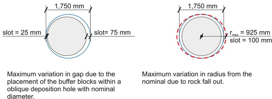
**Figure 4-2.** Possible variations in width of the pellet filled gap between bentonite blocks and deposition hole wall due to different causes of deviations in deposition hole geometry. The scale of the deviations is enlarged with a factor of two.
