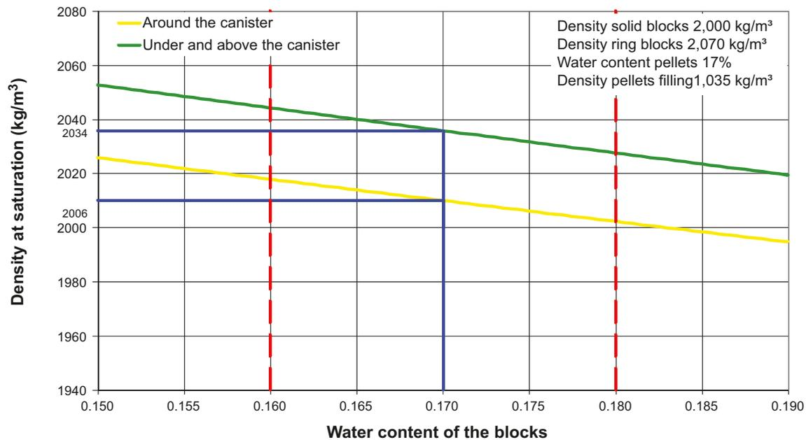
**Figure 4-7.** The calculated saturated density of the buffer as function of the water content of the blocks. The calculations are based on the nominal geometry of the deposition hole, nominal bulk density of the blocks and pellets and nominal water content of the pellets.
