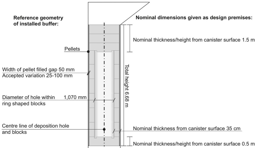
**Figure 3-3.** Reference geometry of the installed buffer and the nominal dimensions given as design premises. Note that the installed dimensions and density will depend on the geometry of the deposition hole. (The upper part of the deposition hole is regarded as part of the deposition tunnel and will be backfilled, see Figure 5-13).
