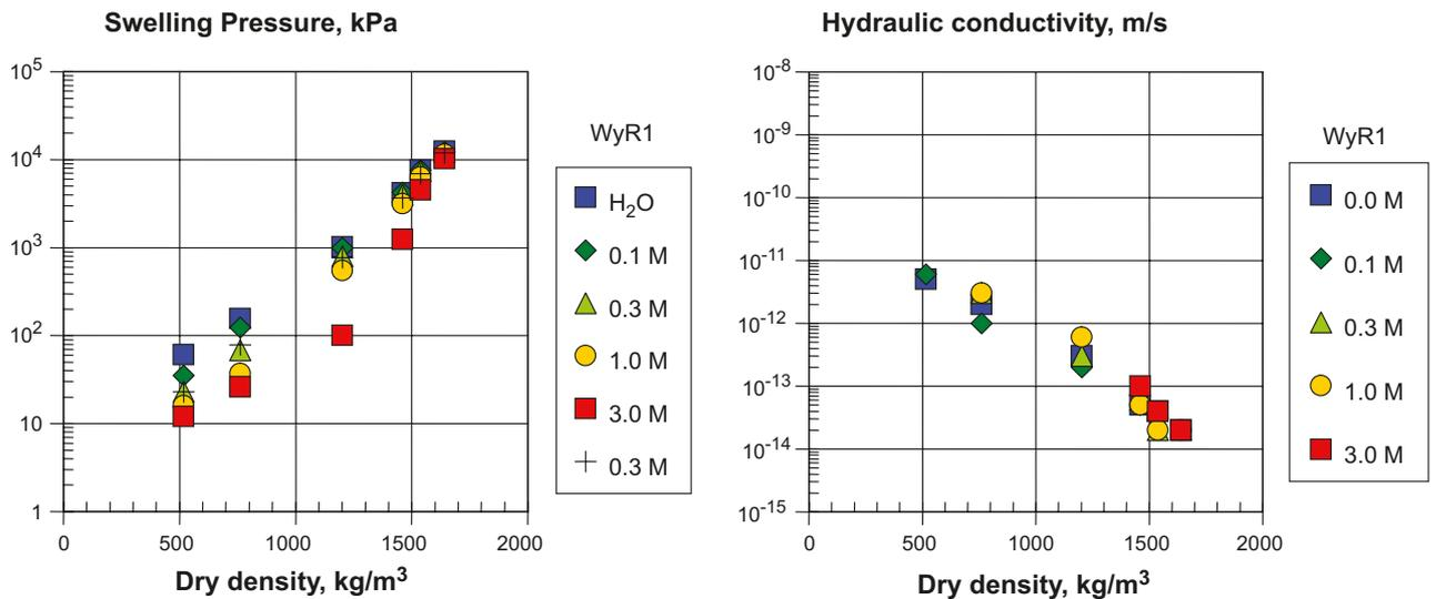
**Figure 4-10.** Swelling pressure (left) and hydraulic conductivity (right) as function of dry density for Wyoming MX-80. The measurements are made with different salt concentrations in the test solution (NaCl) /Karnland et al. 2006/
