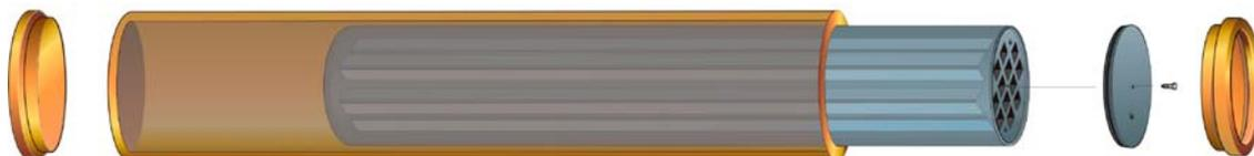
**Figure 3-3.** Exploded view of the reference canister and its components (from the left: copper base, copper tube, insert, steel lid for insert and copper lid).
