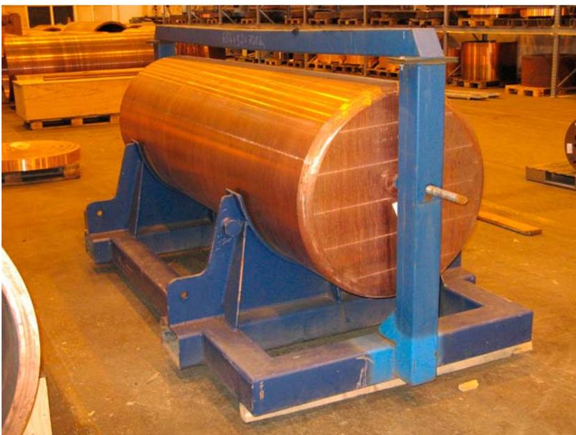
*Figure 5-9. Large copper ingot weighing approximately 12 tonnes.*
