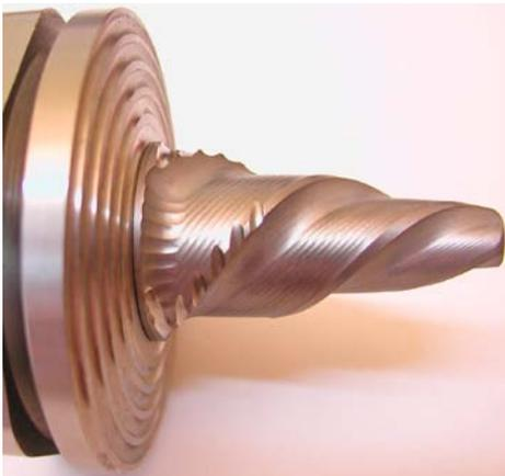
*Figure 5-24. Welding tool.*
