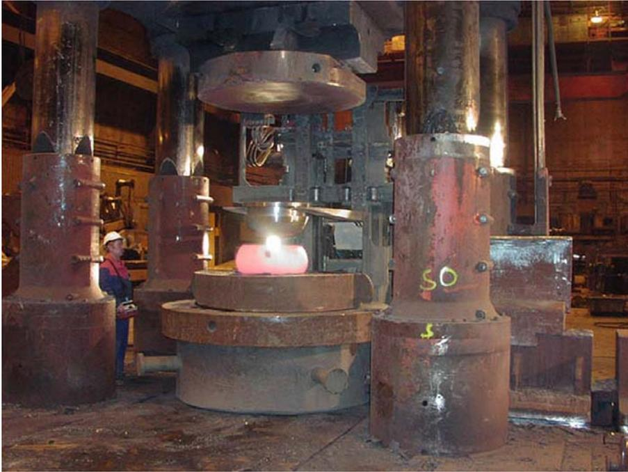
*Figure 5-17. Forging of a lid blank.*
