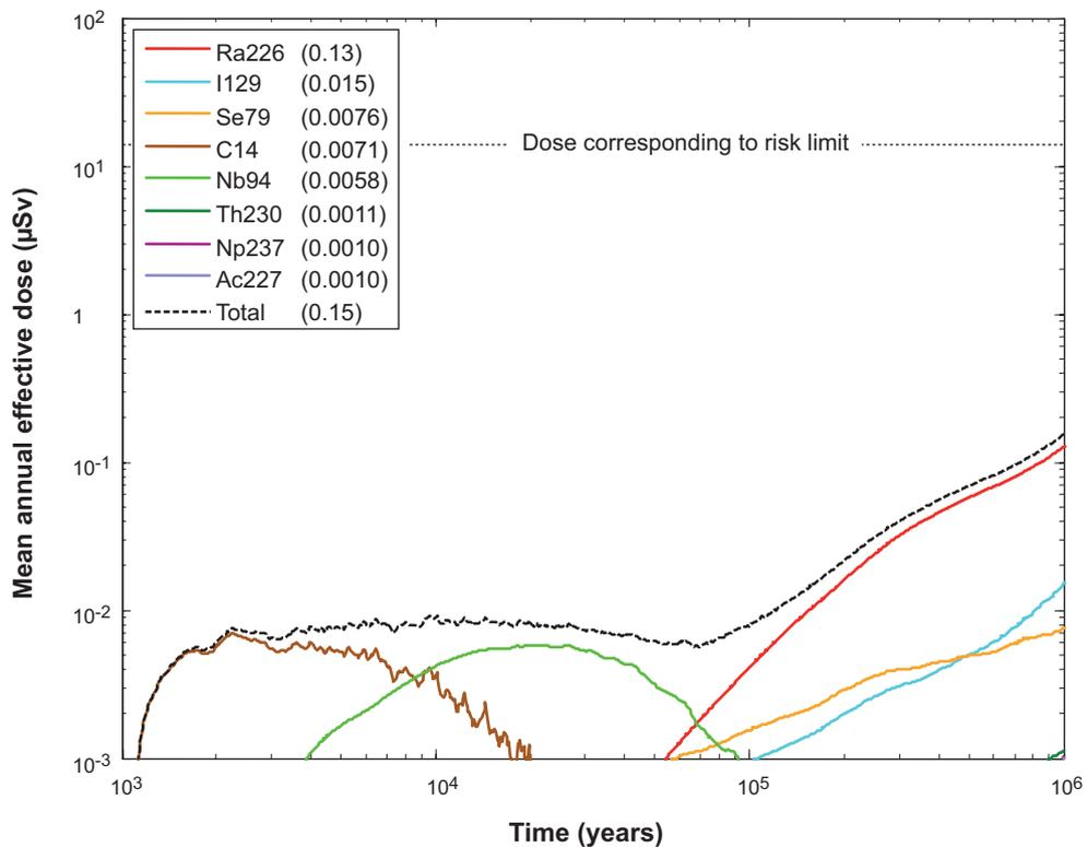
**Figure S-11.** Probabilistically calculated consequences of shear failure, for the period between 1,000 years and one million years. The legends are sorted according to descending peak mean annual effective dose over one million years (given in brackets in  $\mu\text{Sv}$ ).
