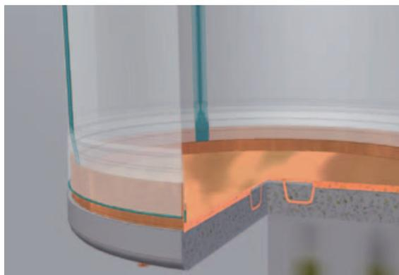
Upper copper plate with fastening devices and a border intended for auxiliary equipment for the installation of the buffer.
