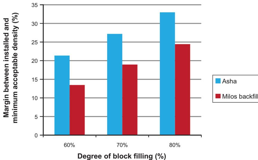
**Figure 5-20.** Margin in ratio between the installed and minimum acceptable density for Milos backfill and Asha and different fractional block filling of the tunnel volume. Calculated from data in the **Backfill production report**, Section 4.4. The margin can be seen as the amount of backfill that could be lost without jeopardising the design premise that the backfill should ensure that the buffer density stays above its designed minimum value.
