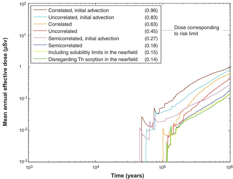
**Figure S-10.** Summary of far-field mean annual effective dose for all probabilistic calculations performed for the corrosion scenario. The peak doses are given in parentheses in  $\mu\text{Sv}$ . In the legend, ‘Correlated’, ‘Uncorrelated’ and ‘Semicorrelated’ refer to three variants of the hydrogeological model used in SR-Site. The three ‘initial advection’ cases put upper bounds on the possible consequences of buffer erosion.
