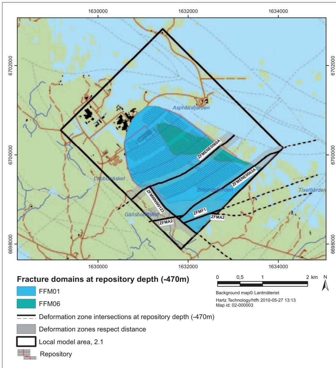
**Figure 5-6.** Reference design layout for the repository at Forsmark, also showing respect distances and the deformation zones requiring the respect distances (Figure 4-1 in the *Underground openings construction report*).
