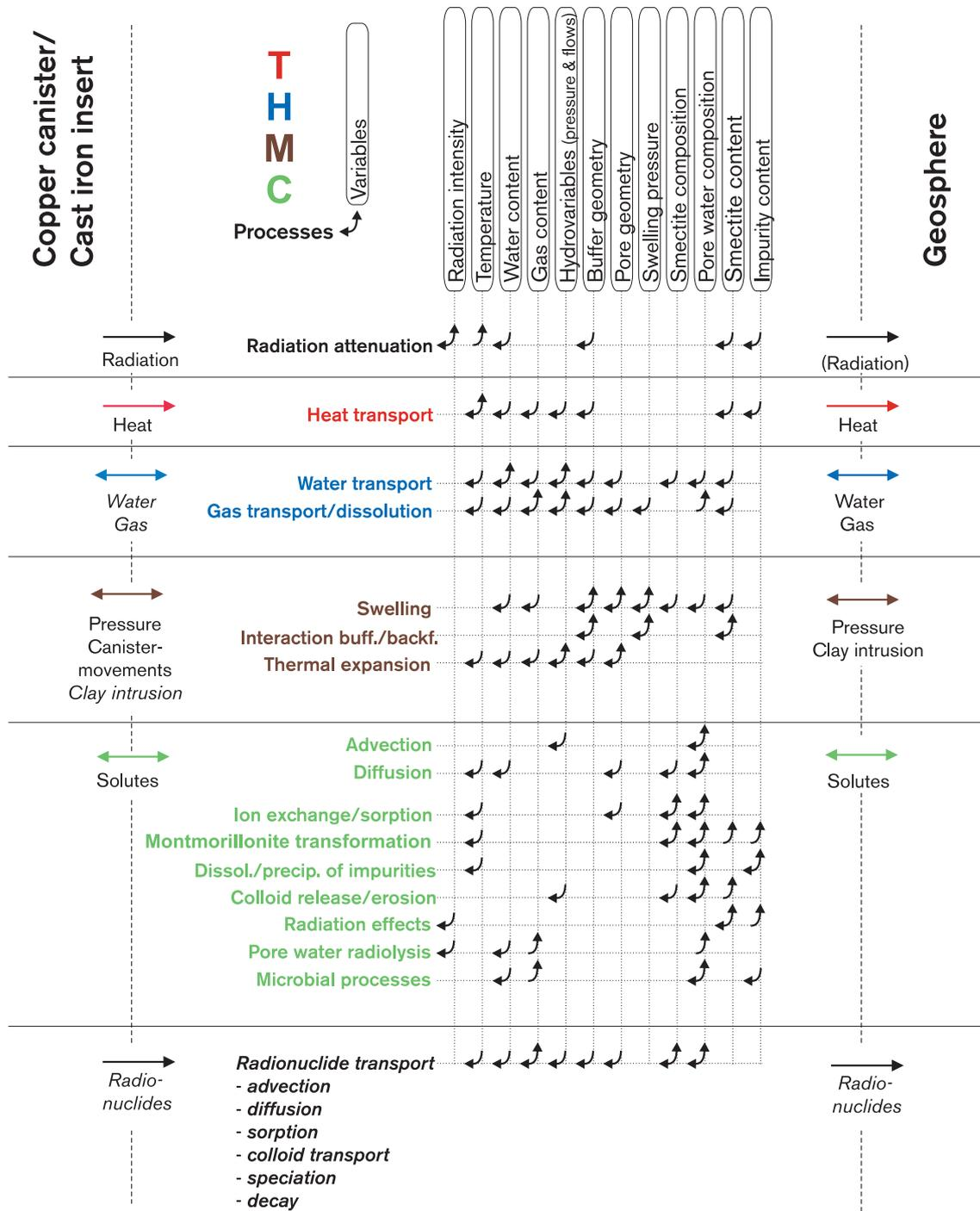
**Figure 7-2.** The SR 97 version of the process diagram for the buffer. Thermal, hydraulic, mechanical and chemical processes are listed in the left column, the variables are given in the top row. Influences between variables and processes are shown by arrows in the diagram. Processes and interactions in italics only occur if containment by the copper canister is lost.
