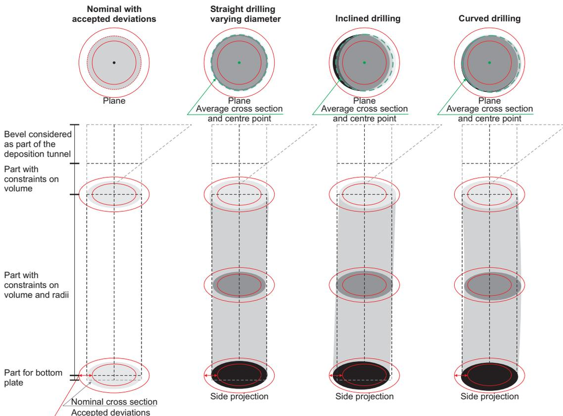
**Figure 5-13.** Some possible causes of deviations in the geometry in a deposition hole without rock fall out. All kinds of deviations can occur in the same deposition hole. The deviations are exaggerated in scale. (The bevel is discussed in the backfilling section).
