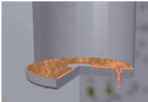
Concrete slab poured through the hole in the centre of the lower copper plate.
