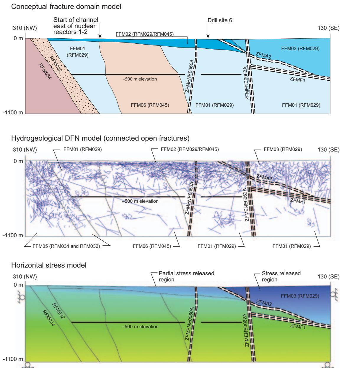
**Figure 4-19.** Comparison of fracture domain, hydrogeological DFN and maximum horizontal stress models along a NW-SE profile in the north-western part of the candidate volume (Figure 11-21 in the *Site description Forsmark*).
