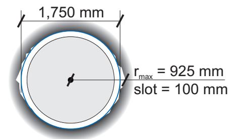
**Figure 5-12.** Increase in deposition hole radius due to spalling and rock fall out in a deposition hole with nominal diameter.
