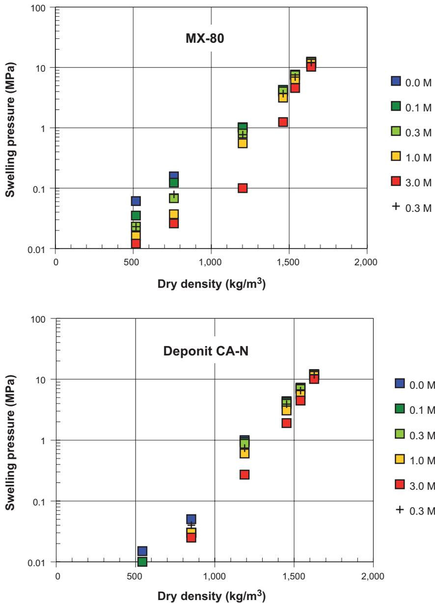
**Figure 5-14.** Swelling pressures of MX-80 exposed to NaCl solutions (upper) and Ibeco RWC (Deponit CA-N) exposed to CaCl<sub>2</sub> solutions (lower). Concentration expressed as M.
