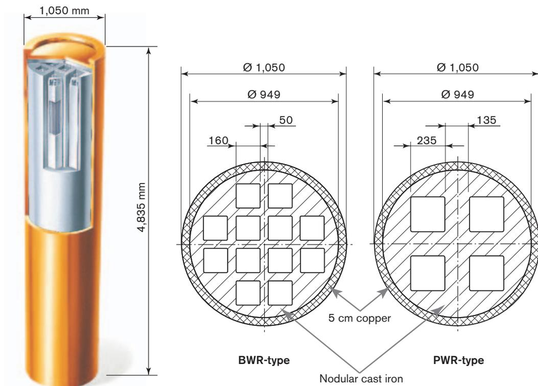
**Figure 5-8.** Left: The reference design with a corrosion resistant outer copper shell and a load-bearing insert of nodular cast iron. Right: Cross section of insert designs of the BWR and PWR types.
