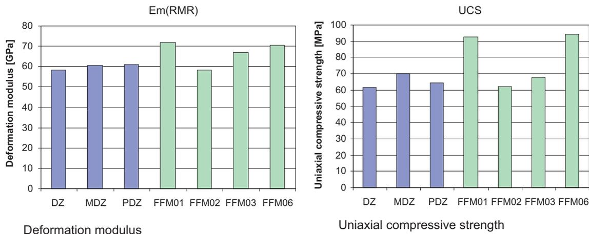
**Figure 4-14.** Mean values of deformation modulus and strength properties of the rock mass in fracture domains and deformation zones as evaluated by an empirical approach (Figure 11-16 in *Site description Forsmark*). DZ = deformation zone, MDZ = minor deformation zone (shorter than 1,000 m), PDZ = possible deformation zone.
