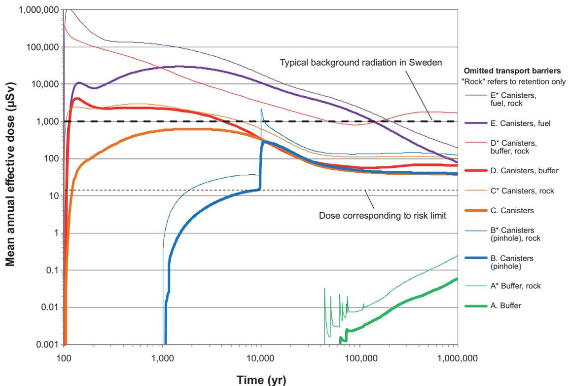
**Figure S-12.** Results of stylised cases to illustrate loss of barrier functions. Note that an omission of the “rock” barrier in these cases refers to omission of retention of radionuclides in the rock fractures only, whereas the favourable, low flow rate at repository depth and the favourable geochemical conditions are still taken into account.
