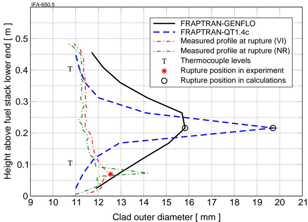
Figure 13: IFA-650.5 rod calculated and measured outer diameter profiles of cladding at burst. The two profiles shown by the solid and dashed lines represent the calculations made by FRAPTRAN-GENFLO and FRAPTRAN-QT1.4c, respectively. The corresponding measured diameter profiles obtained by visual inspection (VI) and neutron radiography (NR) are shown by the dash-dot lines (Oberländer, Espeland, and Jenssen 2008) and maximum measured diameter from VI is marked by asterisk.
