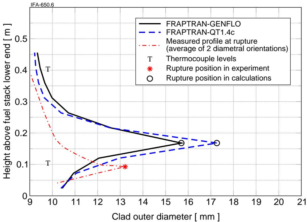
Figure 14: IFA-650.6 rod calculated and measured outer diameter profiles of cladding at burst. The two profiles shown by the solid and dashed lines represent the calculations made by FRAPTRAN-GENFLO and FRAPTRAN-QT1.4c, respectively. The corresponding measured diameter profile is shown by the dash-dot line (Kekkonen 2007b) and maximum measured diameter by asterisk.
