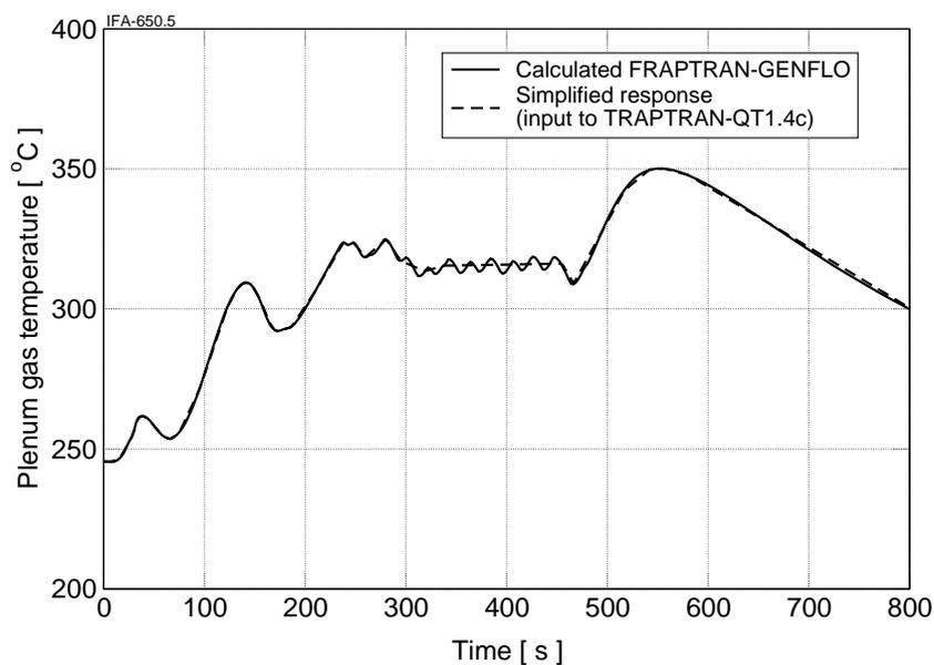
Figure 8: IFA-650.5 / Solid line; FRAPTRAN-GENFLO calculated time variation of plenum gas temperature. Dashed line; Simplified curve of the calculated response. The plenum gas temperature described by the dashed line is prescribed in the IFA-650.5 calculations by the FRAPTRAN-QT1.4c code.
