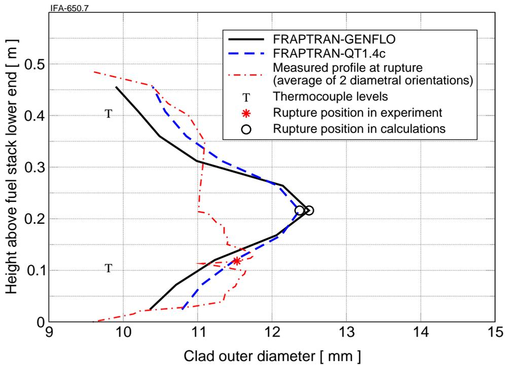
Figure 15: IFA-650.7 rod calculated and measured outer diameter profiles of cladding at burst. The two profiles shown by the solid and dashed lines, respectively, represent the calculation outcome by the FRAPTRAN-GENFLO and FRAPTRAN-QT1.4c codes. The measured diameter along the rod is shown by the dash-dot line (Oberländer, Espeland, Solum, and Jenssen 2008) and maximum measured diameter by asterisk.
