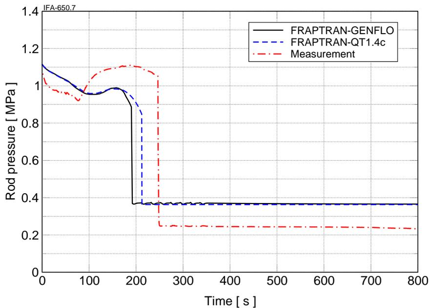
Figure 12: IFA-650.7 rod gas pressure variation with time calculated by the FRAPTRAN-GENFLO and FRAPTRAN-QT1.4c code. The measured rod gas pressure variation during the transient is shown by the dash-dot curve (Jošek 2008).
