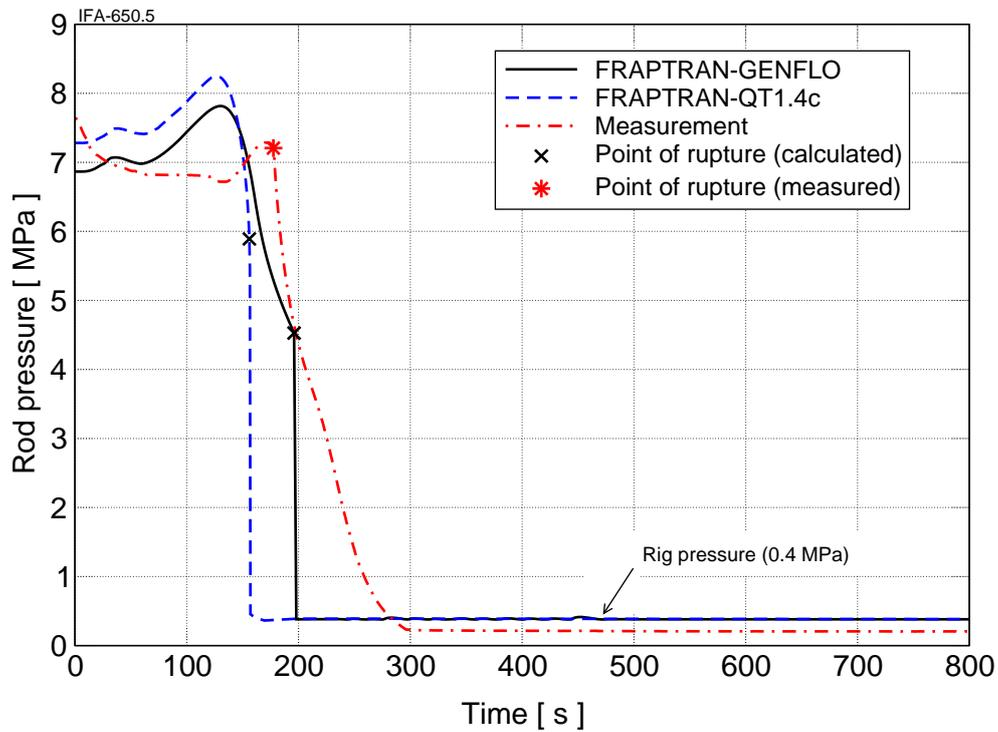
Figure 10: Rod gas pressure (plenum pressure) vs. time for the IFA-650.5 test calculated by the FRAPTRAN-GENFLO (solid line) and FRAPTRAN-QT1.4c (dashed line) codes. Cladding rupture is calculated at 198 and 157 s after start of blowdown, respectively. The measured evolution of the rod pressure is shown by the dash-dot curve. The calculated points of rupture are marked with a star symbol (×) and measured rupture point with an asterisk symbol.
