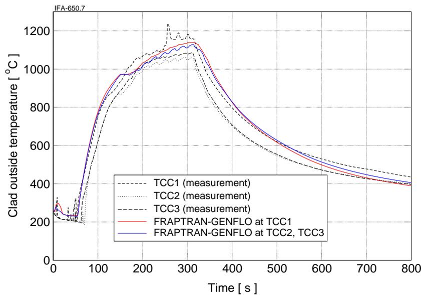
Figure 7: IFA-650.7 / Measured and calculated cladding outer surface temperatures in thermocouple positions. The axial positions of the cladding thermocouples (TCC) for the test are given in table 2. The calculated cladding temperature boundary conditions by FRAPTRAN-GENFLO are prescribed in the calculations by the FRAPTRAN-QT1.4c code.
