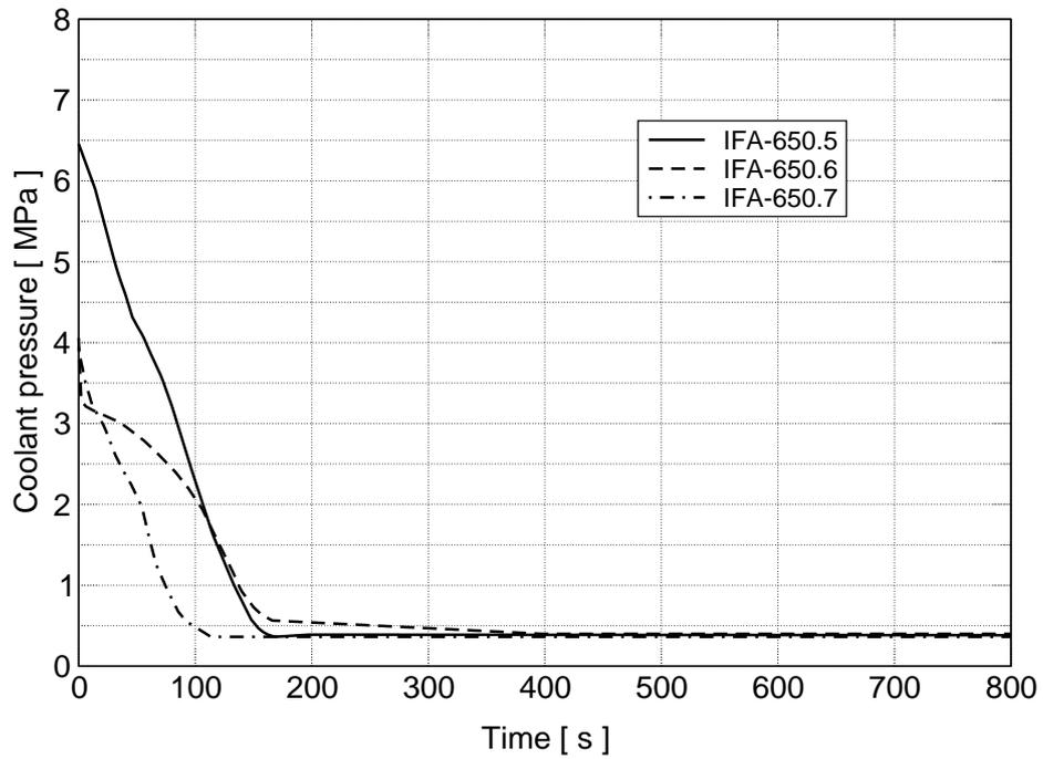
Figure 5: Calculated coolant pressure (rig pressure) variations with time for the IFA-650 tests 5, 6 and 7 using the FRAPTRAN-GENFLO code. The calculated coolant pressure boundary conditions by FRAPTRAN-GENFLO are prescribed in the calculations by the FRAPTRAN-QT1.4c code.
