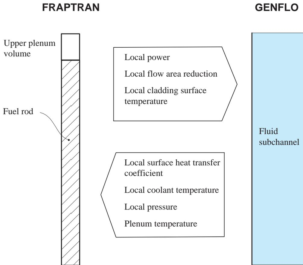
Figure 4: Coupling and data exchange in FRAPTRAN-GENFLO.
