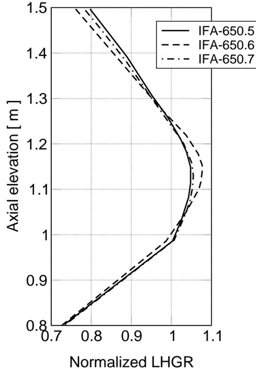
Figure 3: Axial power distributions produced by nuclear fission in the IFA-650.5/6/7 test fuel rods in the Halden reactor. Axial elevation versus normalized linear heat generation rate, adapted from (Kekkonen 2007a; Kekkonen 2007b; Jošek 2008). The lower end of the fuel stack is located at the axial elevation of 0.9 m.
