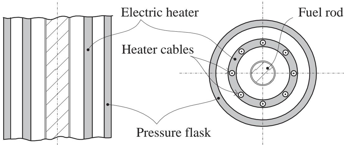
Figure 1: Schematic drawing of the IFA-650 test rig cross sections.
