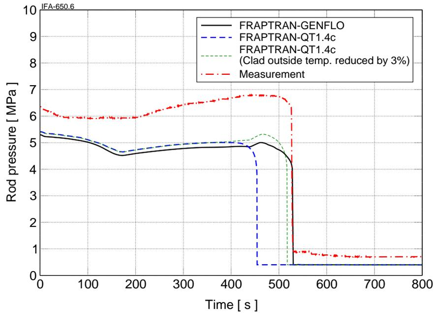
Figure 11: IFA-650.6 rod gas pressure variation with time calculated by the FRAPTRAN-GENFLO and FRAPTRAN-QT1.4c codes. The measured rod gas pressure variation during the transient is shown by the dash-dot curve (Kekkonen 2007b).
