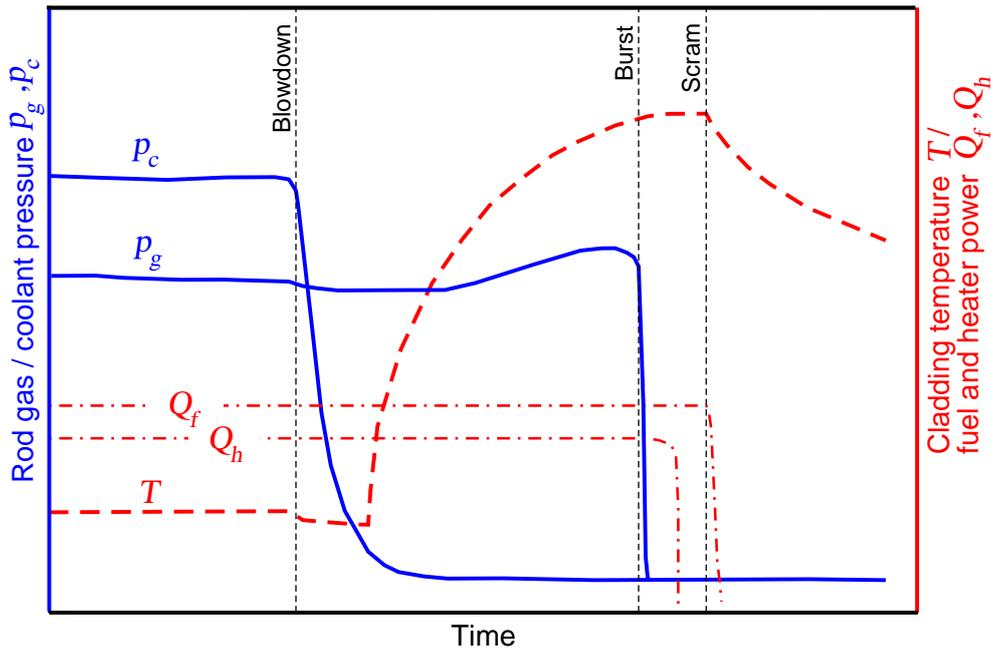
Figure 2: Schematic description of typical time responses of some selected parameters during a Halden IFA-650 LOCA experiment. The LOCA transient (test) is initiated by the blowdown and terminated by reactor scram.
