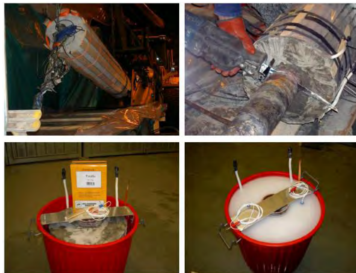
Figure 4.1: Extraction of the LOT A2 test parcel and retrieval of the exposed copper electrodes for further real-time monitoring.
