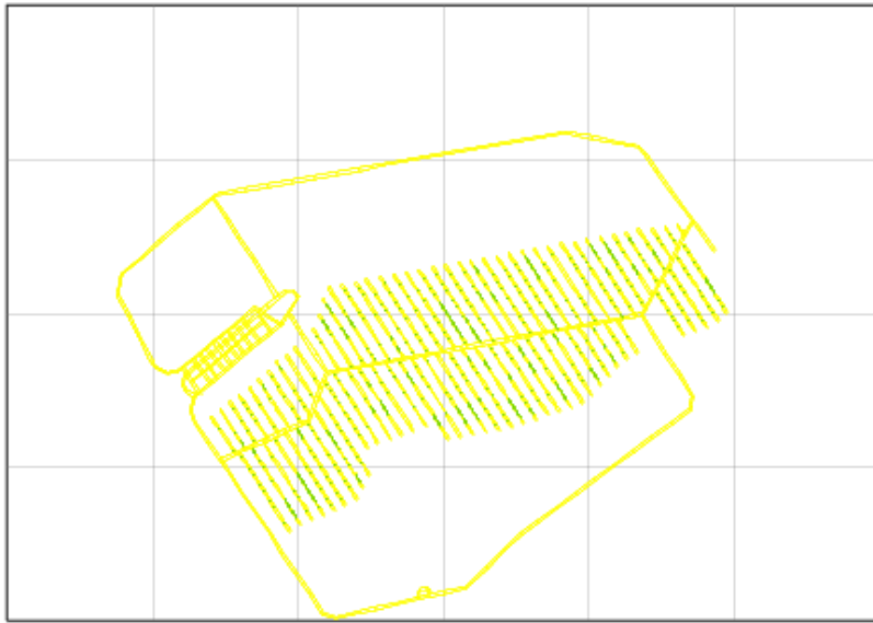
Figure 3.11 Tunnel EDZ features and deposition holes for Forsmark repository Section BD (Base Case Realization 01). EDZ features are indicated in yellow; deposition holes for positions that satisfy the deposition-hole criteria in this realization are in green.
