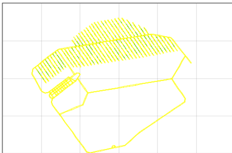
Figure 3.10 Tunnel EDZ features and deposition holes for Forsmark repository Section AC (Base Case Realization 01). EDZ features are indicated in yellow; deposition holes for positions that satisfy the deposition-hole criteria in this realization are in green. The grid (grey lines) is a reference grid with 1 km spacing(see caption of Figure 3.7 for explanation).
