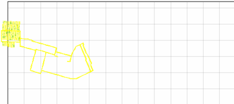
Figure 3.3 Tunnel EDZ features and deposition holes for Laxemar repository Section D (Base Case Realization 01). EDZ features are indicated in yellow; deposition holes for positions that satisfy the deposition-hole criteria are in green.
