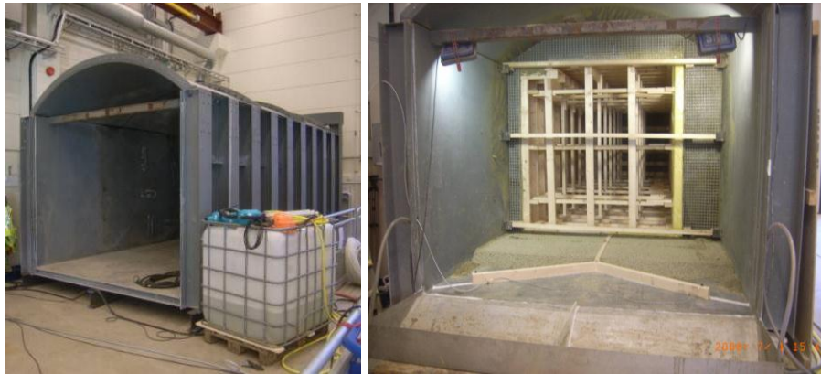
Figure 4_14. Photographs of a half-scale backfill test. Bentonite backfill was emplaced as pre-compacted bentonite blocks inside a half scale tunnel mock up (left). A wooden former (right) was used to reduce the total amount of backfill needed for the test as compared with the repository situation. Spaces between the tunnel wall and the bentonite blocks were filled with bentonite pellets. Water was injected into the backfill at various rates through holes in the tunnel walls (SKB R-08-132).
