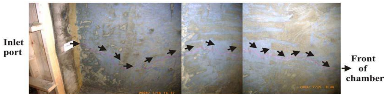
(b) Test 12 showing flow path along wall of chamber
