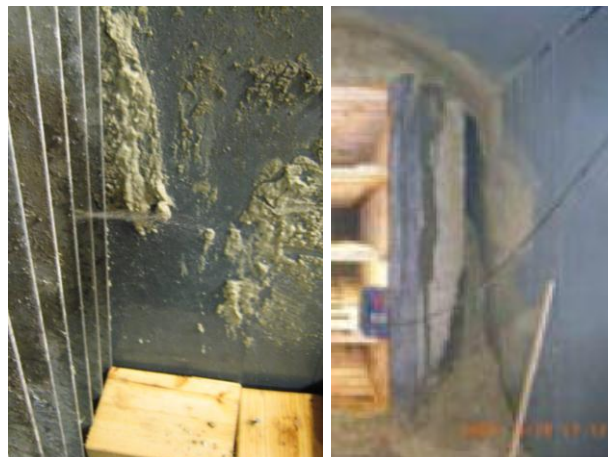
Figure 4_15. Photographs of water spraying out from the front surface of the backfill test (left) and the erosion of bentonite pellets (right) illustrating the effect of piping, channelled flow and erosion (SKB R-08-132).
