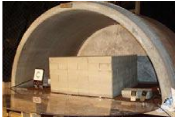
Figure 4_11. Blocks of compressed Friedland clay stacked inside a concrete tunnel (SKB R-08-134).
