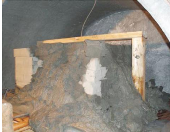
Figure 4_12. The effect of dripping water on unconfined blocks of compressed Friedland clay (SKB R-08-134).
