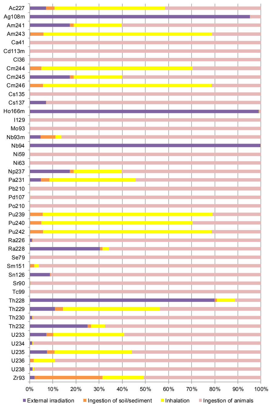
Figure 26: Contribution of different exposure pathways to the maximum dose factor for adults in the pasture system for each radionuclide.
