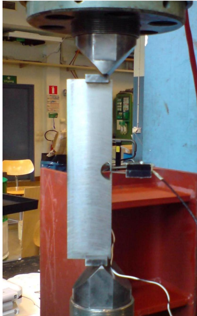
Figure 3.1: Experimental setup of pre-loading of test specimen.
