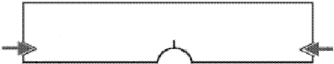
Figure 2.1: In-plane compression of notched test specimen.
