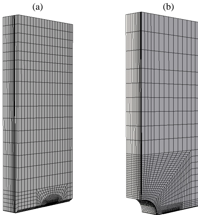
Figure 0.21. Three dimensional finite element mesh for (a) a quarter model of the side-grooved three point bending specimen, (b) a quarter model of the un-grooved notched three point bending specimen.
