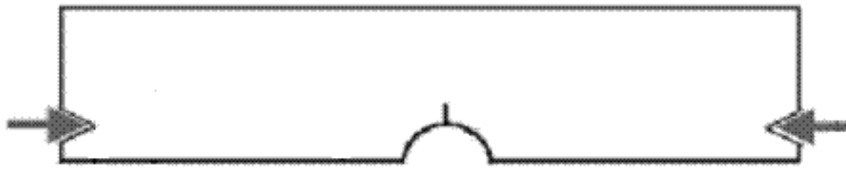
Figure 0.28. In-plane compression of the notched test specimen.
