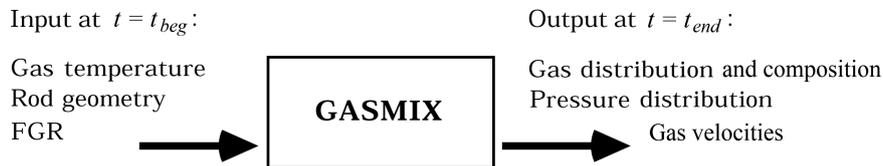
**Figure 4:** Purpose of the GASMIX subroutine. Here,  $t_{beg}$  and  $t_{end}$  refer to the time at beginning and end of a global time step in FRAPCON or FRAPTRAN.
