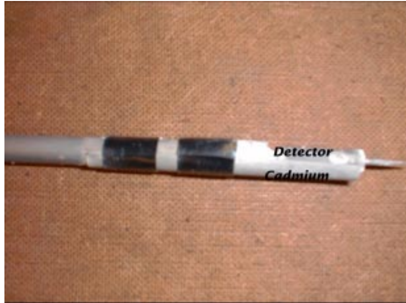
Fig. 1. Photo Showing the Construction of the Fibre Detector, Measuring the Partial Current, With One Half Covered With Cadmium
