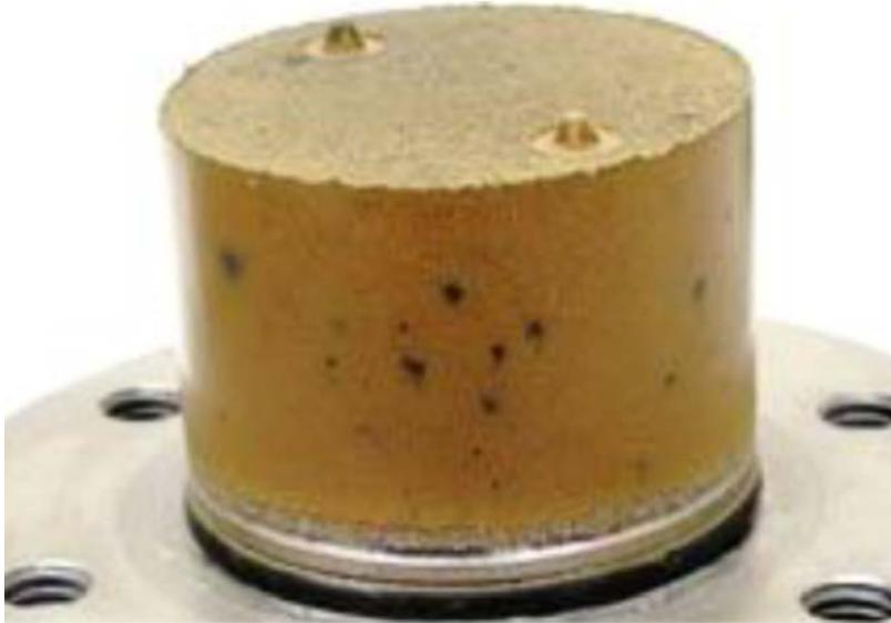
Black colonies of iron sulphide produced by sulphide producing bacteria in Asha bentonite at 1750 kg/m<sup>3</sup> wet density and with addition of lactate and sulphide producing bacteria
