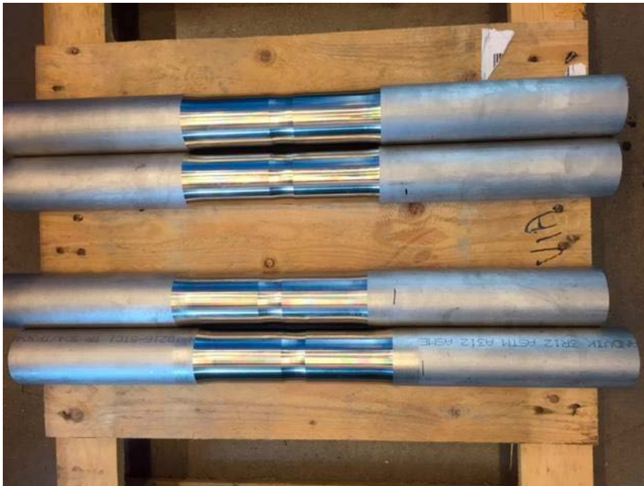
Figure 3. Different test specimens after machining and prior to welding the lids at the extremities.
