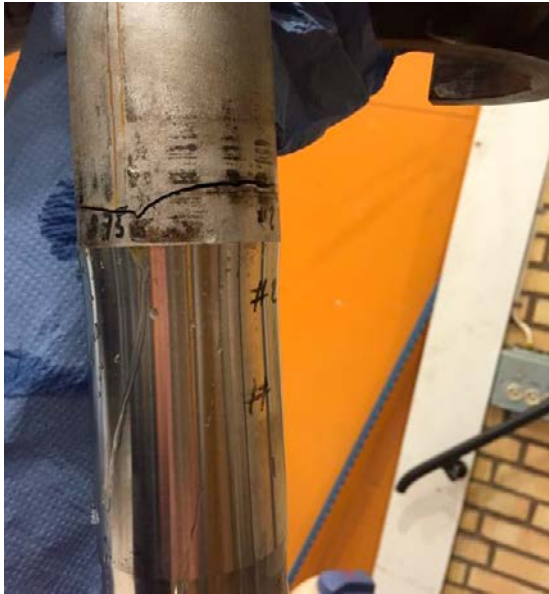
Figure 10. Failure of pipe 2 below a clamp of the fixture due to fretting fatigue.
