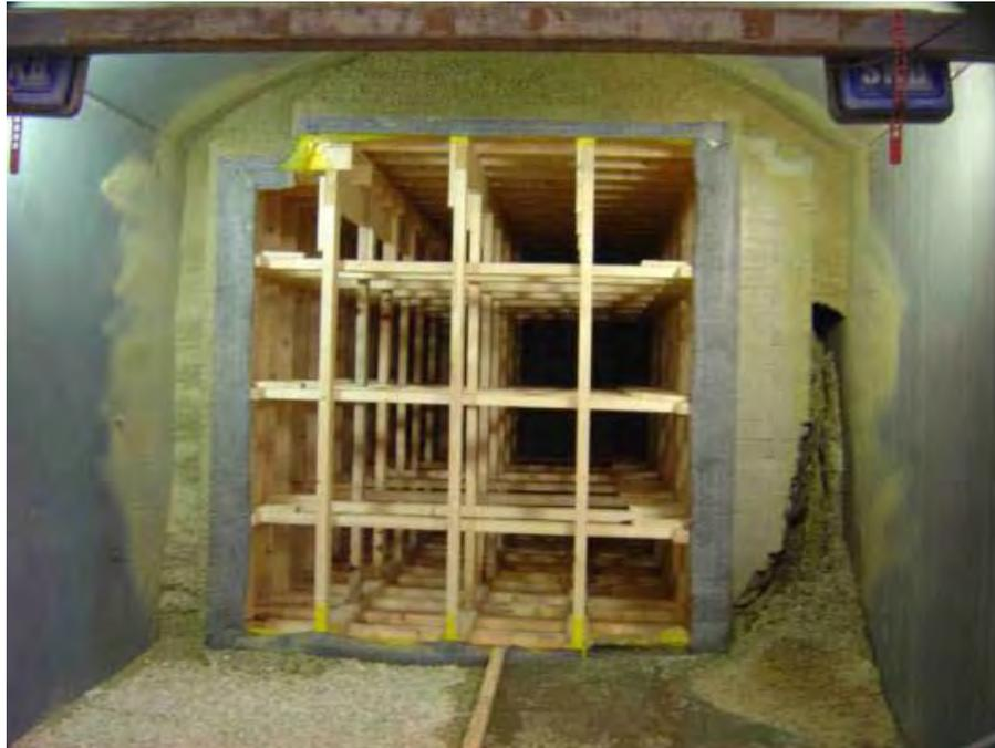
**Figure 2.6** Photograph of a 1/2-scale backfilling test performed at the Äspö hard rock laboratory showing backfill erosion caused by water inflow and movement in channels or pipes (from Dixon *et al.* 2011b).
