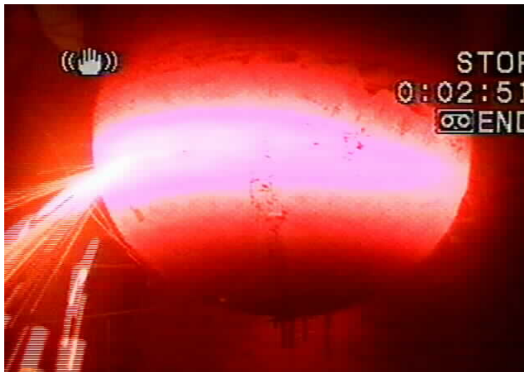
Figur 2.4.1: Tryckkärlsbrott i EC-FOREVER 3(b) test.
