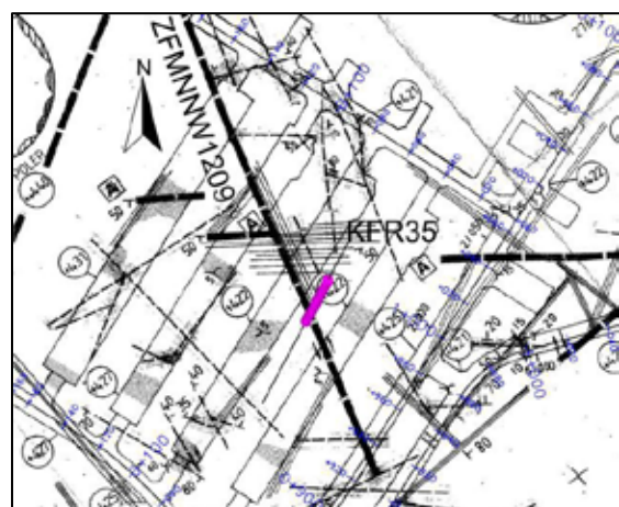
ZFMNNW1209 crossing the rock caverns and intercepted by KFR35 as it appears in the model (left) and the original overview mapping /Christiansson and Bolvede 1987/. The zone is modelled with a thickness of 18 m based on KFR35 SHI.
