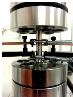
Figure 5-7 A close-up photo of the specimen, specimen fixture and extensometers.
