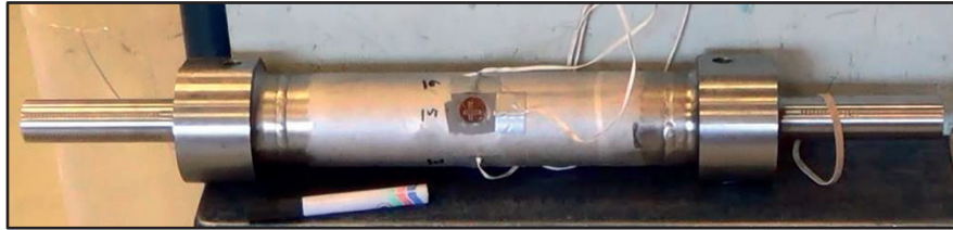
Figure 6-5 Photo of a 316L test specimen and a marker pen.
