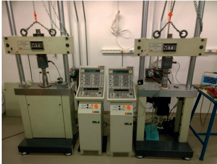
Figure 5-4 Two-rod experimental setup with two test machines.
