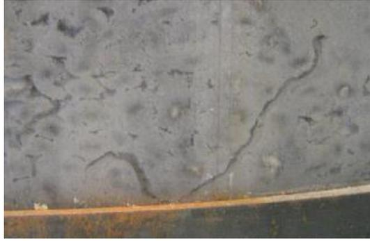
**Figure 2.13** A channel formed by piping in the pellet-filled outer part of the buffer (from R-09-29).
