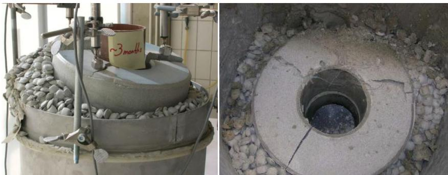
**Figure 2.16** Heaving and cracking of MX-80 buffer rings, and partial wetting of MX-80 bentonite pellets after 3 months of inflow at 0.0001 litres/minute, equivalent to ~0.5 litres/year<sup>1</sup> (from R-10-70).
