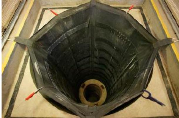
**Figure 2.6** Buffer water protection sheet (from TR-10-15)
