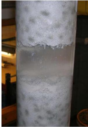
**Figure 2.15** Photograph of bentonite pellets in a tube that have been displaced by water pressure (from R-10-70).
