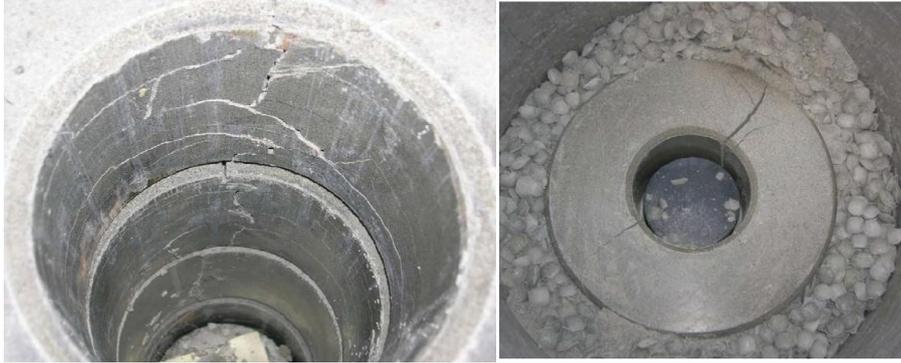
**Figure 2.17** Cracked MX-80 bentonite rings (from R-10-70). The figure on the right shows the result from a test involving hydration of MX-80 bentonite blocks and pellets at a low water inflow rate of 0.00001 litres/minute, equivalent to ~5 litres/year<sup>1</sup>. The buffer is seen to have cracked in a radial fashion and the pellets have not hydrated uniformly (from R-10-70).
