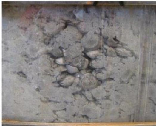
**Figure 2.14** Heterogeneous wetting of the pellet-filled outer part of the buffer. Almost intact pellets can be seen after 7 days of water inflow (from R-09-29).
